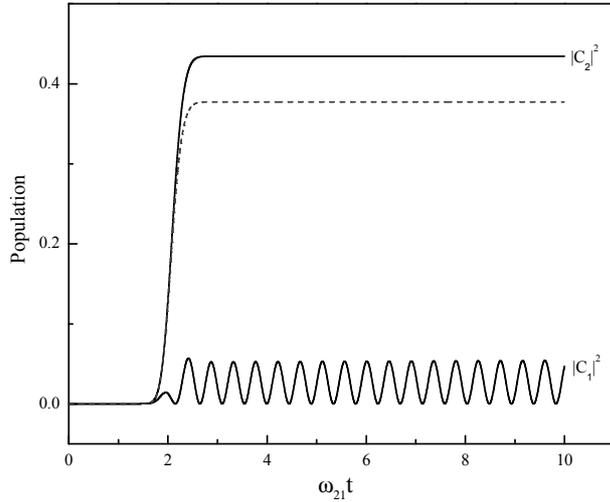
Figure 4.8: Populations of the atomic states 1 and 2 for  $\Omega_c = 5\omega_{21}$  and  $r_1 = r_2$ . In the absence of coupling field, the populations of the states 1 and 2 are equal (dashed gray line).
