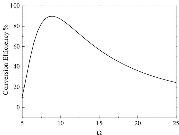
Figure 3.2: Quantum efficiency of optical field conversion from  $\lambda_1 = 795\text{nm}$  into  $\lambda_2 = 780\text{nm}$  in  $^{87}\text{Rb}$  as a function of driving field Rabi frequency  $\Omega$  (given in units of  $\Gamma_2$ ) for the medium length  $L = 100\mu\text{m}$ . For the rest of parameters see the text.
