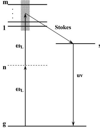
Figure 4.11: Level scheme of atoms illustrating two-photon excitation of a manifold of upper structure containing  $m$  atomic eigenstates and generation of the Stokes and UV fields on the basis of hyper-Raman scattering and four-wave mixing, respectively.
