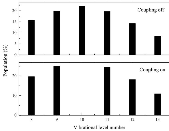
Figure 4.4: Histogram of the vibrational population distribution after excitation without (upper frame) and with (lower frame) the coupling field.
