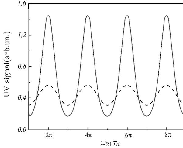
Figure 4.12: The UV signal obtained from Eq.(4.54) as a function of time delay  $\tau_d$  for a model atoms having two upper eigenstates with the energy difference  $\hbar\omega_{21}$  (solid). The parameters are chosen such that at the minima of  $|f(t)|^2$  the condition (4.55) is violated, while at the maxima the exponential gain (4.56) takes place. The QB in  $|f(t)|^2$  is shown by dashed line.
