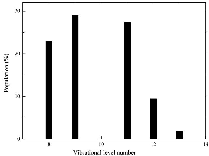
Figure 4.5: Histogram of the vibrational population distribution after excitation by the same pulses used in Fig. 4.4 but of duration 600 fs.
