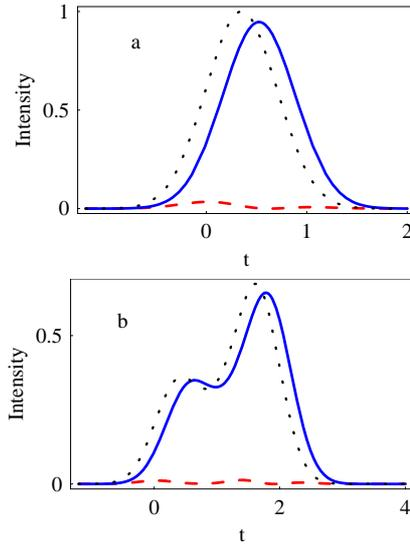
Figure 3.3: Output shapes of  $\lambda_1$  (dashed line) and  $\lambda_2$  (solid line) modes in the cases of Gaussian (a) and double-hump (b) input  $\lambda_1$  pulses for  $\Omega = 8\Gamma$  and other parameters as in Fig.3.2. The dotted line displays the  $\lambda_1$  pulse propagating in the medium with  $\beta = 0$ . The time is given in units of  $T$ .
