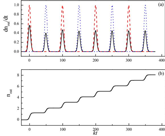
Figure 2.5: Flux (a) and total number (b) of output cavity photons versus the time (in units of  $k^{-1}$ ) generated on the cycling transition  $5S_{1/2}(F = 2) \rightarrow 5P_{3/2}(F' = 3)$  in  $^{87}\text{Rb}$  atom. The atom is initially in the state  $|F, -F\rangle$ . The laser subpulses have a duration  $T = 0.5\mu\text{s}$  and the same delay time as in Fig.2.4.
