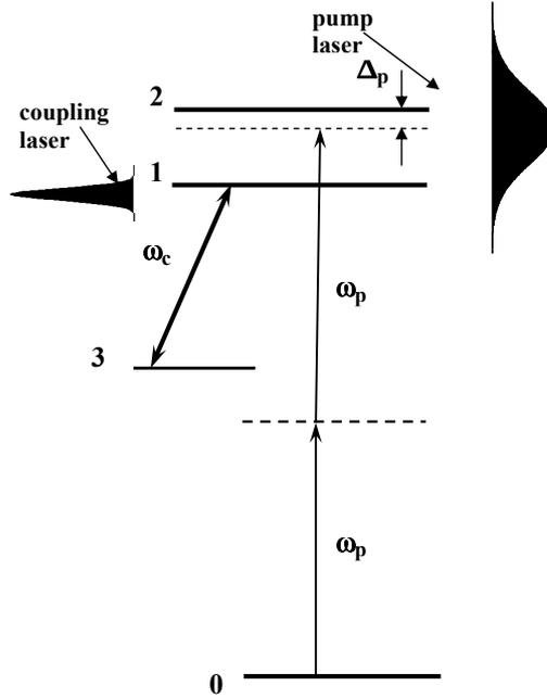
Figure 4.7: Level scheme of model atom illustrating two-photon excitation of two upper eigenstates by ultrashort pump laser and interaction with coupling field on the auxiliary transition  $1 \rightarrow 3$ .
