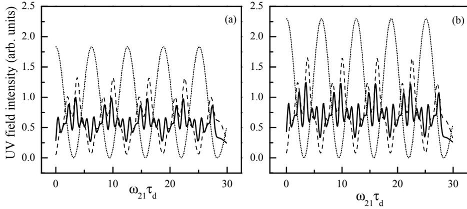
Figure 4.17: Dependence of intensity of UV field on delay time between pump and probe pulses  $\tau_d$  in arbitrary units. Dotted line -  $\Omega_c = 0$ , dashed line -  $\Omega_c = 3\omega_{21}$ , solid line -  $\Omega_c = 5\omega_{21}$ .  $\mathcal{E}_{pr}/\mathcal{E}_p = 0.7$ , (a)  $r_2/r_1=1$ , (b)  $r_2/r_1=0.5$ .
