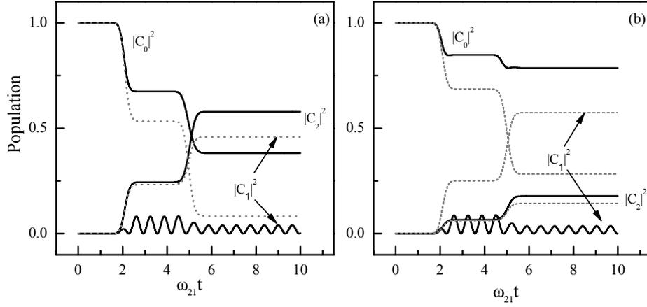
Figure 4.16: Population of the atomic levels 0, 1, 2 in the presence ( $\Omega_c = 5\omega_{21}$ ) and absence of coupling field - solid and dashed lines, the pump and probe pulses are turned on at the moments  $\omega_{21}t_p = 2$  and  $\omega_{21}t_{pr} = 5$ , respectively.  $\mathcal{E}_{pr}/\mathcal{E}_p = 0.7, \omega_{21}\tau_d = 3$ , (a)  $r_2/r_1 = 1$ , (b)  $r_2/r_1=0.5$ .
