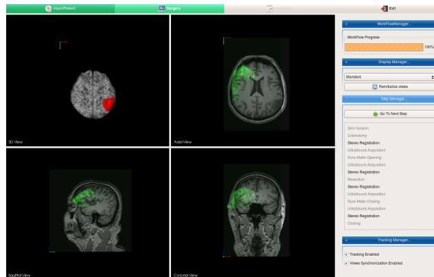
Figure 2.2: Visualization of the intraoperative application. The acquired ultrasound image is overlaid in green on top of the pre-operative MR image.
