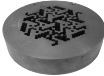
Figure 2.3 – Rank-6 HURA tungsten collimator: thickness: 12 mm, hole-to-hole distance: 1.85 mm
