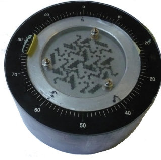
Figure 3.49 – ZnSn coded collimator
