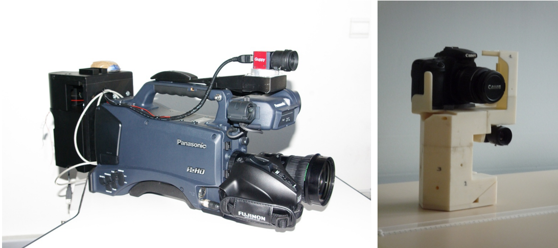
Figure 3.9: The Gyroviz project: Coupling an image acquisition device with a set of inertial sensors. Left: Video camera coupled to a FOG, GPS and Guppy TM camera. Right: Still camera coupled to a FOG and Guppy TM camera.
