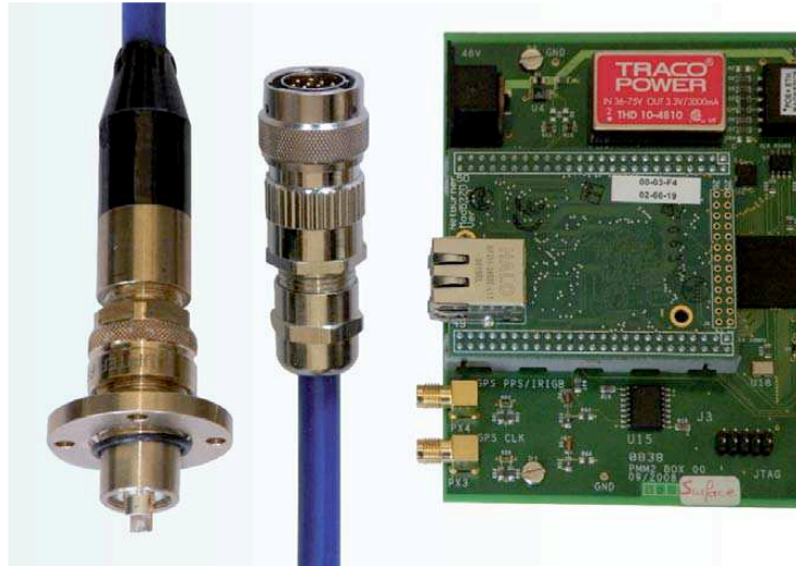
Figure 1.20. The surface card and an example of the cable and watertight connector.
