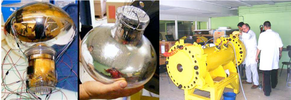
Figure 1.19. Left: the 12-inch PMT equipped with strain gauges and PMT with broken glass because of the pressure. Right: the vessel for the pressure tests shipped from BNL laboratory.
