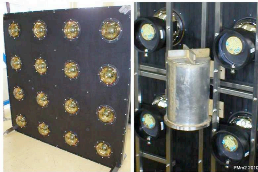
Figure 2. Large demonstrator realized by the IPNO with 16 \times 8 -inch Hamamatsu tubes. On the right the back of the PMTs with the waterproof enclosure that contains the front-end card.
