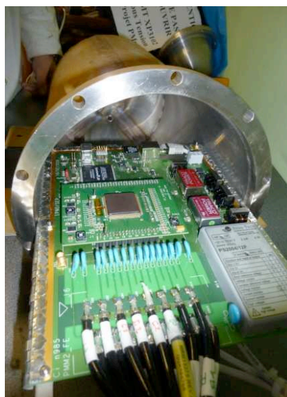
Figure 1.18. The waterproof enclosure realized to place the front-end under water.
