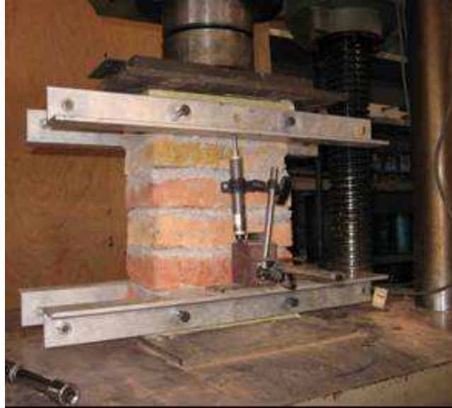
Figure 4.18: Experimental setup for compression test
