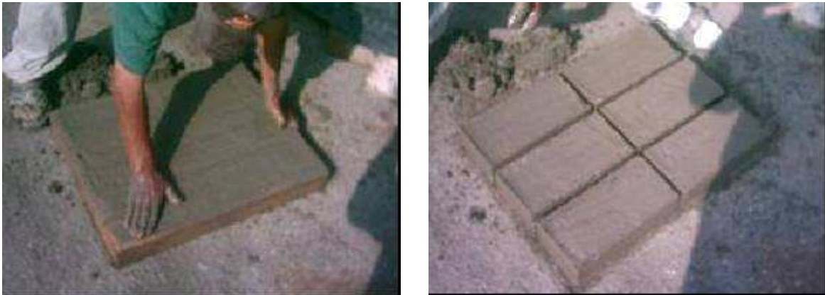
Figure 2.3: Manual process to obtain solid clay bricks
