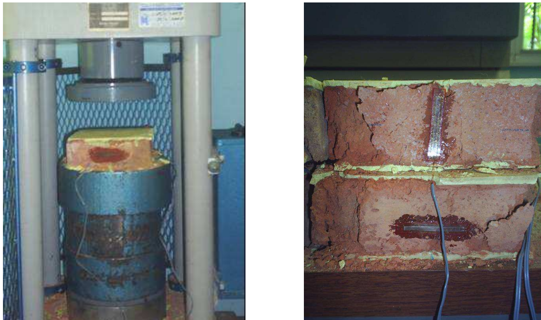
Figure 4.1: Experimental setup of compressive test on solid clay bricks and tested specimen
