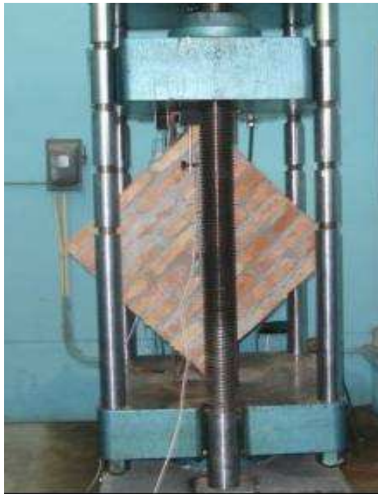
Figure 4.7: Experimental setup of diagonal tension test
