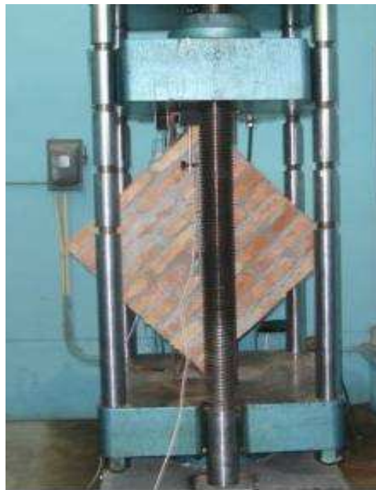
Figure 4.7: Experimental setup of diagonal tension test
