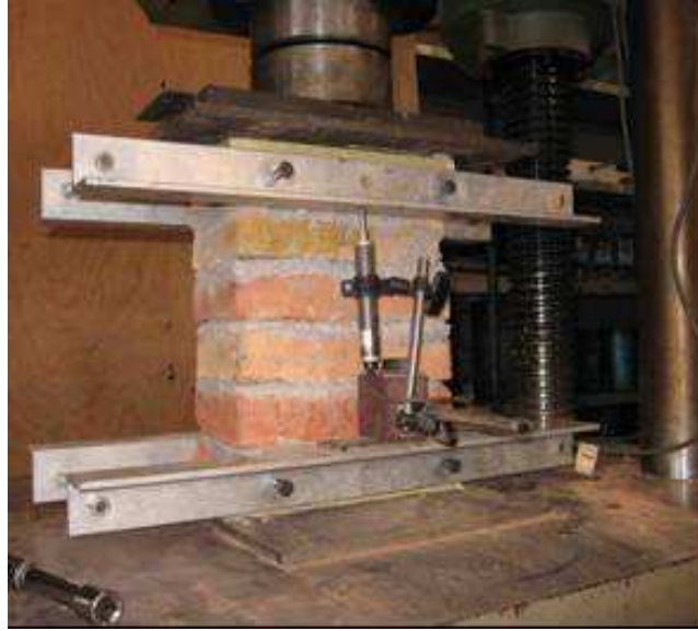
Figure 4.18: Experimental setup for compression test
