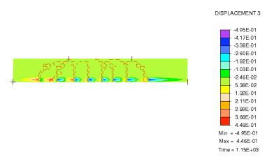
Figure 3.8: Cracks pattern and bond slip sliding
