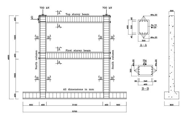
Figure 1.12: RC frame diagram in computation and experiment
