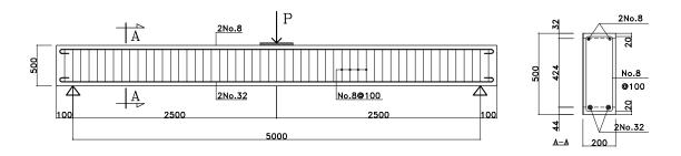
Figure 1.9: Reinforced concrete beam in computation
