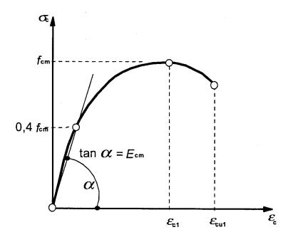
Figure 2.2: Stress-strain curve of concrete in compression of experiment
