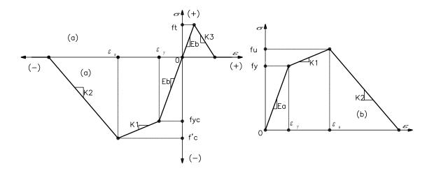
Figure 2.8: Material behaviors of concrete and reinforcement
