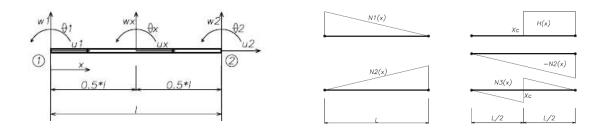
Figure 1.5: 2D bar element and shapes of the interpolation functions
