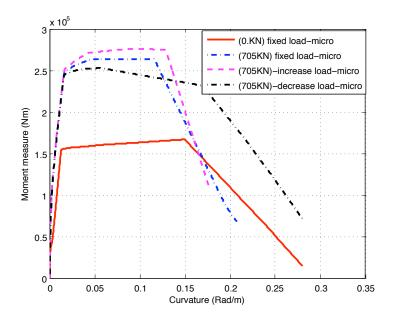
Figure 2.25: Multi-fiber computation for reinforced concrete single-element console
