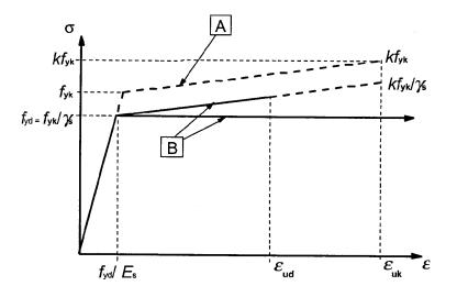
Figure 2.1: Stress-strain curve of steel for design
