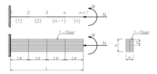
Figure 2.6: Imposed axial load and rotation in multi-fiber and stress-resultant beamcolumn element
