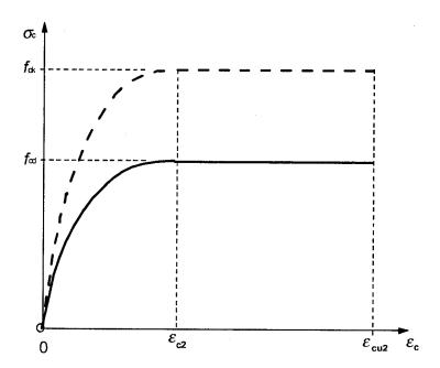
Figure 2.4: Parabolic-rectangular curve in compressive zone of bending beam
