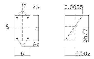
Figure 2.3: Ultimate strains in members under compression
