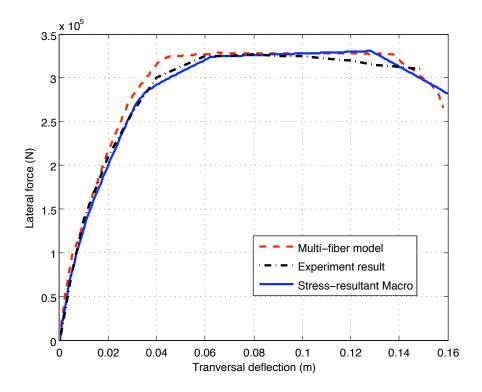
Figure 1.16: Relation of lateral load versus deflection at top storey of frame
