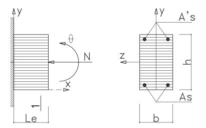
Figure 2.9: Multi-fiber beam-column diagram for parameter identification
