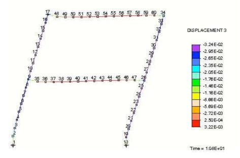
Figure 1.15: Rotational displacement of frame
