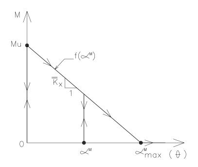
Figure 1.3: Moment-rotation behavior at the discontinuity point of beam element
