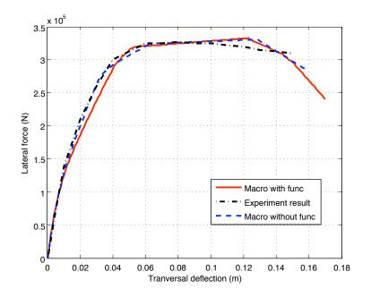
Figure 2.39: Transversal load and deflection in frame
