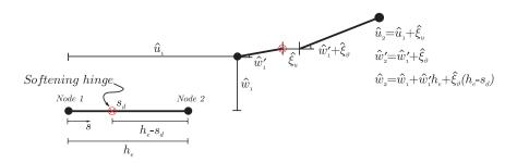
Figure 1.1: Displacement discontinuities in the Euler-Bernoulli beams
