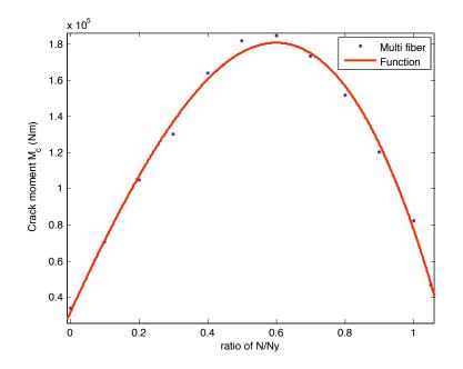
Figure 2.17: Best-fit function for cracking moment  $M_c$  variation with respect to n= N/Ny
