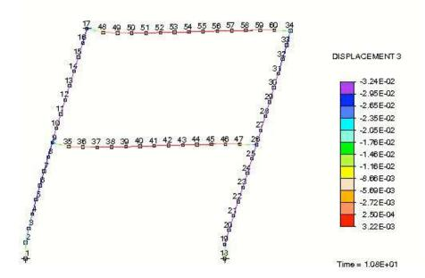
Figure 2.38: Rotation displacement of frame in computation
