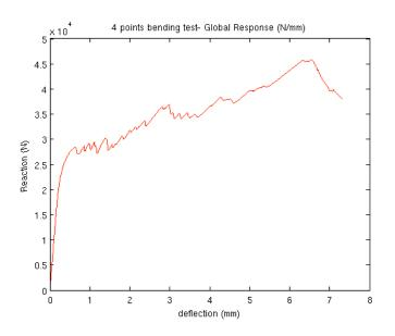
Figure 3.6: Global response for the heavy reinforcement
