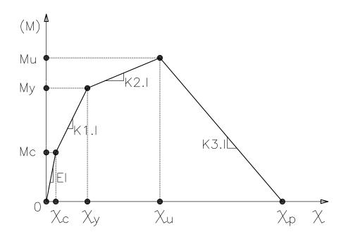
Figure 2.7: Stress-resultant macro model for frames
