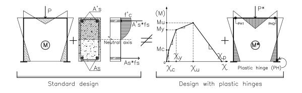
Figure 1: Standard design procedure and performance based design procedure
