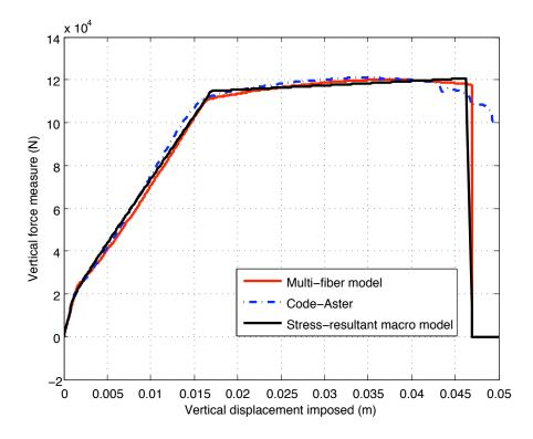
Figure 1.11: Relation of reaction and vertical displacement
