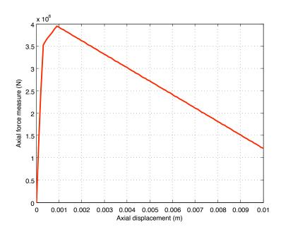
Figure 2.11: Axial force identification for rectangular cross-section
