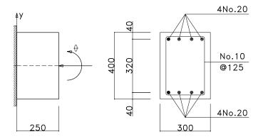
Figure 2.10: Geometry of reinforced concrete built-in beam-column for parameter identification
