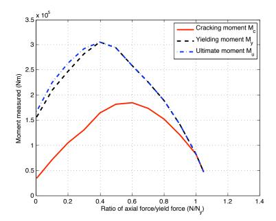
Figure 2.15: Cracking, yielding and ultimate moments with respect to N/Ny ratio
