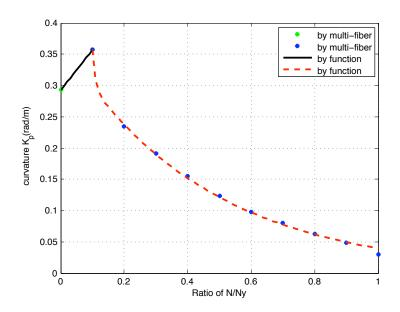
Figure 2.23: Best-fit function for curvature at rupture point  $\kappa_p$  variation with respect to n=N/Ny
