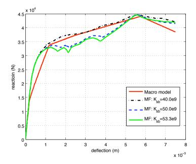
Figure 3.16: Global behavior of support reaction and deflection of tested beam
