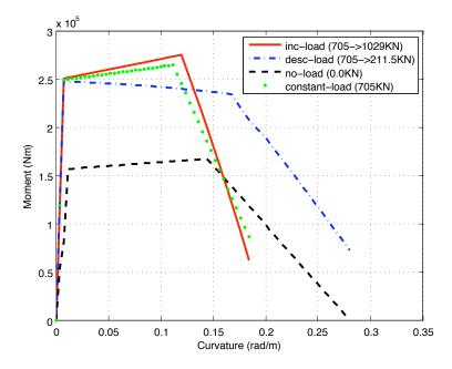
Figure 2.26: Stress-resultant beam macro computation for reinforced concrete single-element console
