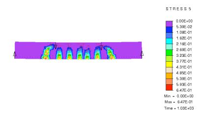
Figure 3.7: Cracks opening in the RC specimen
