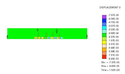
Figure 3.3: Bond-slip along the bar and crack pattern for the first macro-cracks
