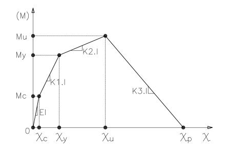
Figure 1.6: Moment-Curvature relation for stress resultant macro model
