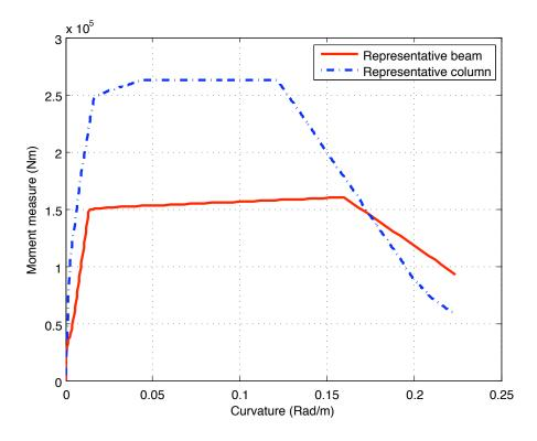
Figure 1.14: Relation of moment-curvature for representative beam and column
