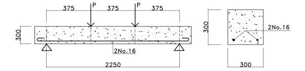
Figure 3.14: Geometry and details of beam in the four-point bending test
