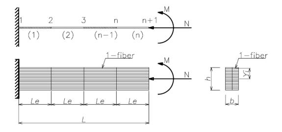
Figure 1.7: Considered beam and fibers in the element
