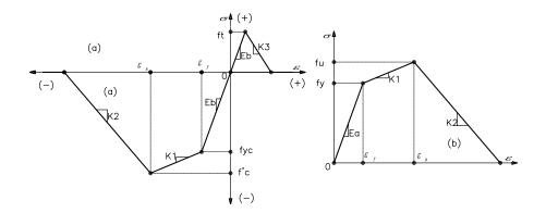
Figure 1.8: Behaviors of concrete and steel
