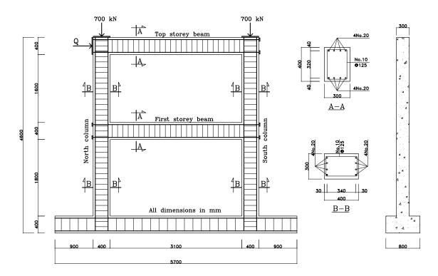
Figure 2.37: Detail of two-storey reinforced concrete frame
