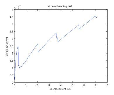
Figure 3.9: Global response for weak reinforcement
