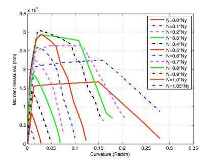
Figure 2.12: Moment-curvature relations obtained by multi-fiber beam-column model based computations
