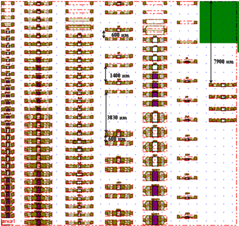
Figure 4.4 General view for all of devices in one die
