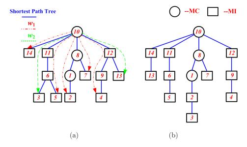
Figure 1.6: (a) Illustration of the Reroute-to-Source Algorithm (b) Illustration of the Reroute-to-Any Algorithm
