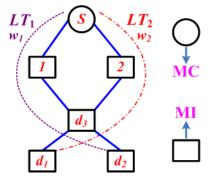
Figure 4.1: An Example Sparse Splitting WDM Network
