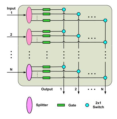
Figure 1.3: The Architecture of a Splitter-and-Delivery (SaD) Switch [34, 91]
