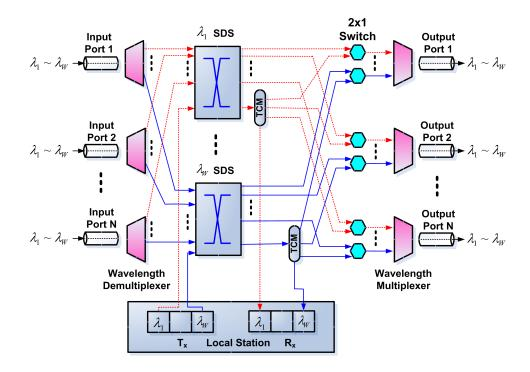
Figure 1.4: The Architecture of a Tap-and-Continue (TaC) OXC [3]
