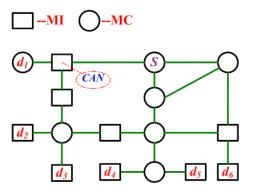
Figure 2.6: An Example Network with CAN Nodes
