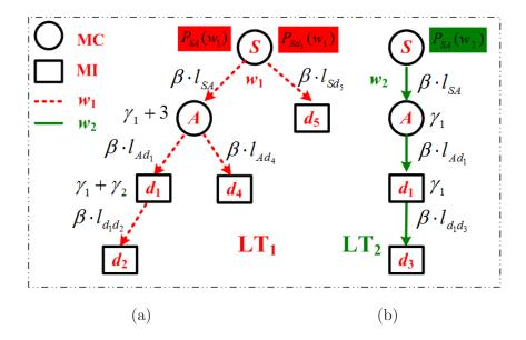
Figure 3.1: Illustration of Power Loss in the Light-Forest for Multicast Session  $ms(s, (d_1 - d_5))$  (a) Light-Tree One (b) Light-Tree Two
