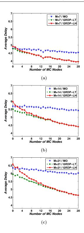
Figure 5.6: Comparison of the Average Delay in the USA Longhaul Topology when Multicast Member (a) Ratio = 25%; (b) Ratio = 50%; (c) Ratio = 75%.
