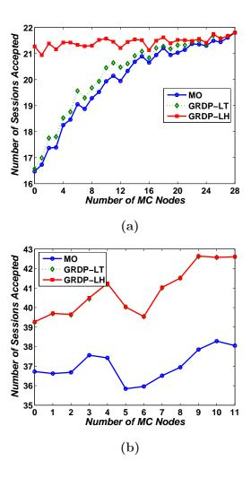
Figure 5.9: Comparison of Throughput in (a) USA Longhaul Topology; (b) Cost-239 Topology.
