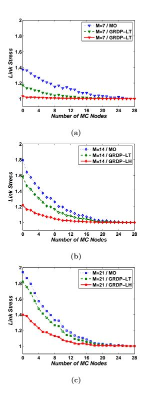
Figure 5.5: Comparison of the Link Stress in the USA Longhaul Topology when the Multicast Member (a) Ratio = 25%; (b) Ratio = 50%; (c) Ratio = 75%.
