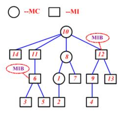
Figure 2.3: The SPT for  $m_1$  Constructed by the Dijkstra Algorithm
