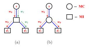
Figure 1.5: The Functionality Difference Between an MI and an MC Node in a Light-Tree
