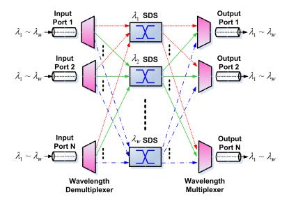
Figure 1.2: The Architecture of a Simple OXC
