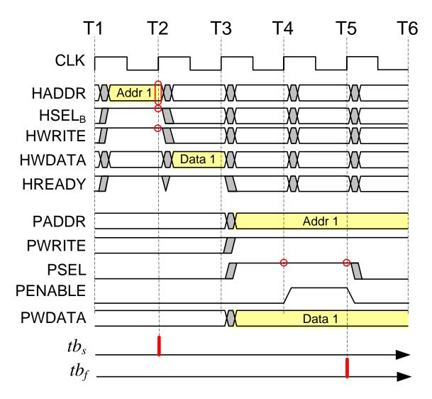
Figure 8.1: A typical write transfer through the bridge
