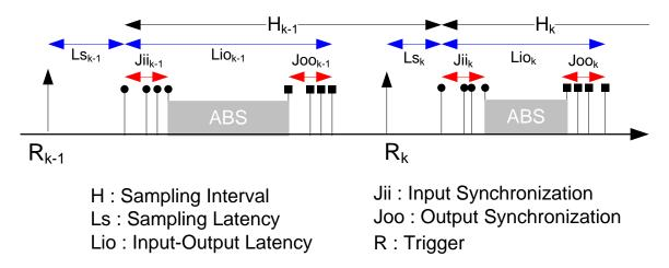
Figure 4.2: Timing requirements for the ABS
