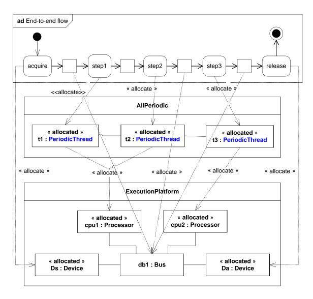
Figure 5.2: Three-layer approach with Marte
