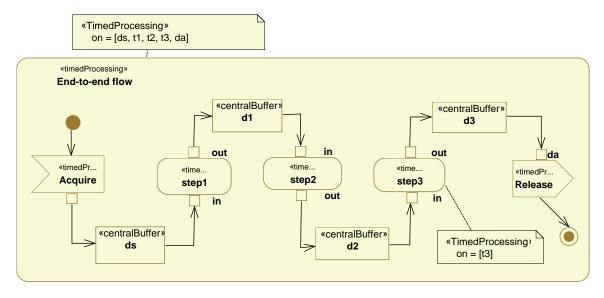
Figure 5.4: End to end flows with UML Marte
