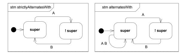
Figure 3.4: CCSL alternatesWith encoded as an automaton
