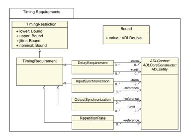
Figure 4.1: The metamodel of East-ADL Timing Requirements.
