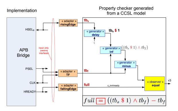
Figure 6.1: The observation network structurally reflects the CCSL model
