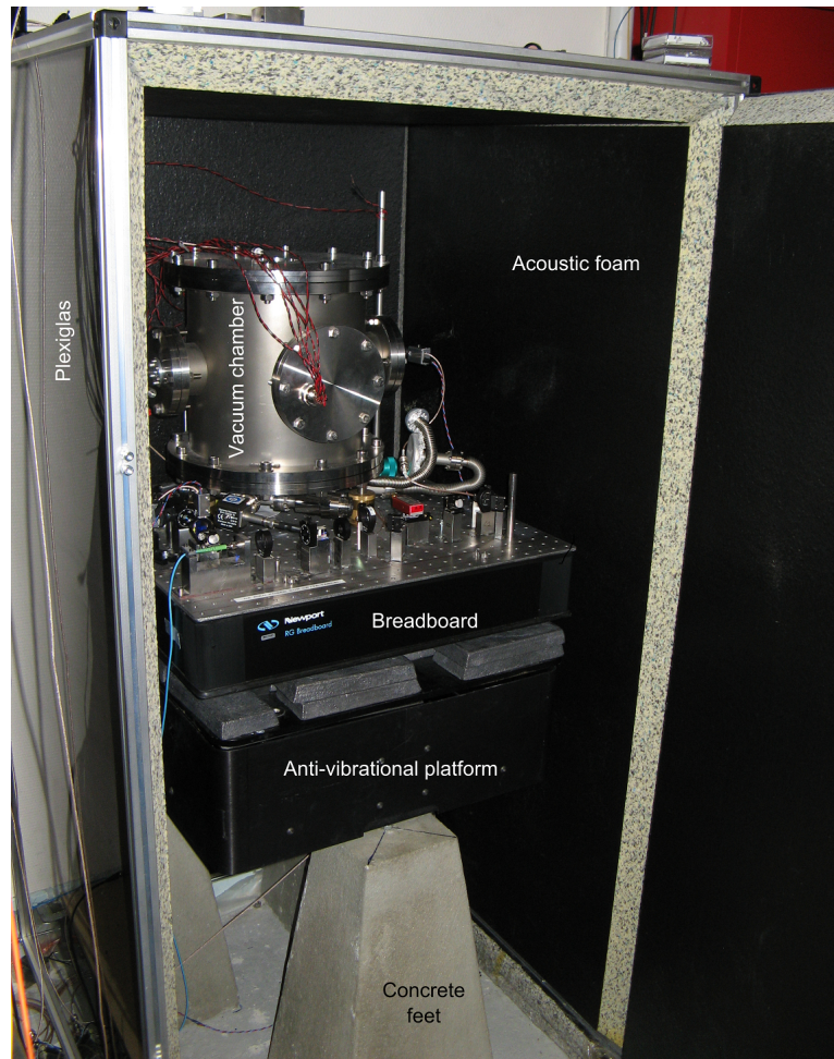
Figure 4.8: The box surrounding the vacuum chamber with the cavity. The vacuum chamber along with the optics needed for mode matching of the light is placed on a breadboard, which rests on an anti-vibrational platform. The platform is supported by three large concrete feet. Under normal operational conditions the door in the right part of the picture is closed.
