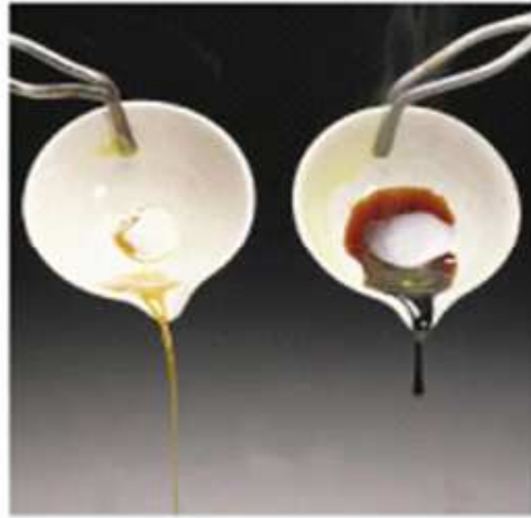
FIGURE 3.14: Liquid sulfur below (left one) and above (right one) the \lambda transition.
