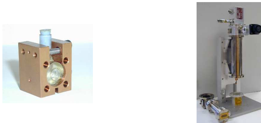
FIGURE 4.8: Sample holder (left) and cryostat (right) used for the IXS measurements on glassy sorbitol.
