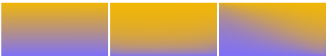
Figure 3.25 Left: Standard diffusion (equal strength), Middle: Orange stronger than blue. Right: Varying strength along curve.
