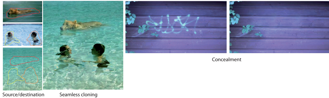
Figure 3.14 Images from Poisson Image Editing by [PGB03] showing application of the Poisson Equation. Left: Seamless cloning. Right: By importing seamlessly a piece of the background undesirable artifacts can easily be hidden.
