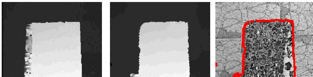
(a) BP results without cooperative boundary extraction (b) Disparity map using proposed approach (BP) (c) Object boundary with 4.13(b)
