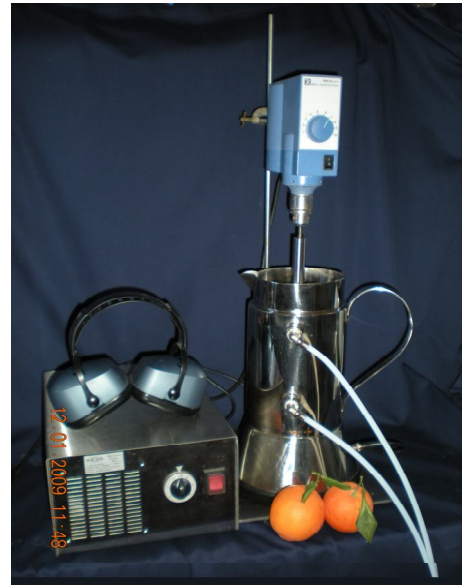
Figure 1: Sonication apparatus used for UAE
