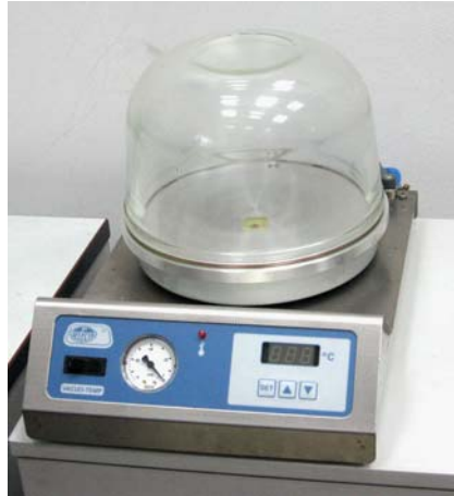
Fig.6.6: Photograph of Vacuo Temp 4000474 climatic chamber of Selecta Company used for thermal aging reliability tests
