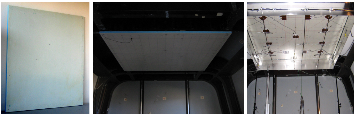
Figure 1.1: Trim panel (left), VASCo cabin with trim panel (middle) and test set up for vibroacoustic control (right)
