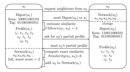
Figure 2.16: Estimating scores in gossip
