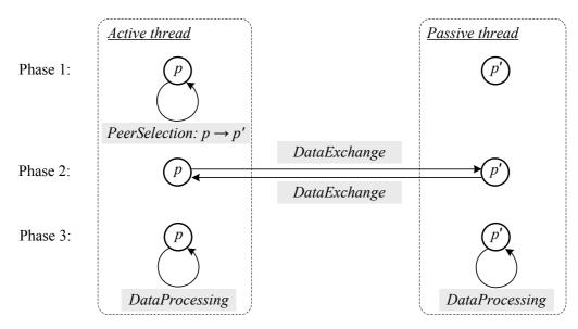
Figure 1.2: A gossip operation between two peers
