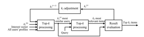
Figure 3.3: Adjusting the personal network  $(k_1)$
