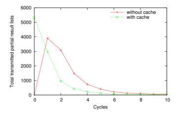
Figure 3.24: Transmission of partial result lists
