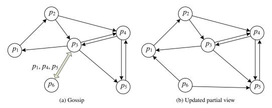
Figure 1.3: Example of gossip-based topology management
