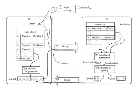
Figure 2.17: Query processing in eager mode (1st cycle)
