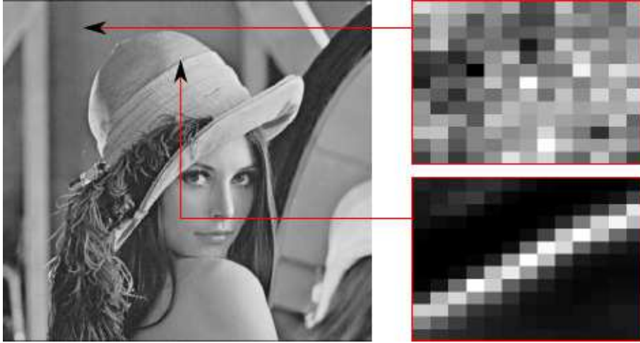
Figure 6.1: Adaptation of the NL-Means kernel to the local structures. The two right images show the kernel weights (\lambda_{\mathbf{x},\mathbf{x}'}_{\mathbf{x} \in \Omega_R(\mathbf{x})}) restricted to a small searching zone \Omega_R(\mathbf{x}) of size R \times \mathbb{R} (with centered on \mathbf{x} ), obtained for a patch in a uniformly regular zone and a patch centered on an edge.
