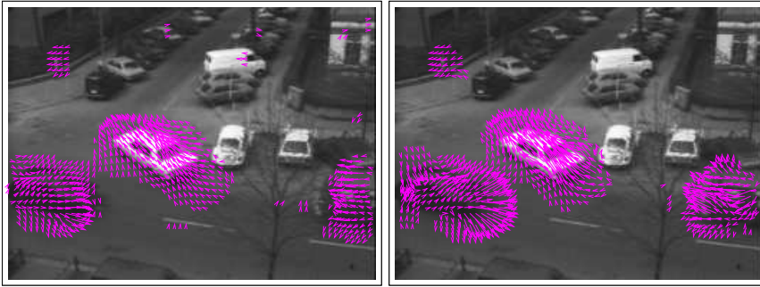
Fig. 3 Comparison Data Assimilation (left) / Horn-Schunk (right) – frame 9.
