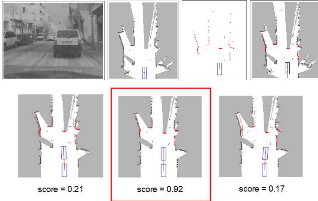
FIGURE 2.7 – Example of scan matching result. From left to right : reference image ; local map created so far M_{t-1} and previous vehicle pose x_{t-1} ; laser scan at time t ; and matching result is obtained by trading off the consistency of the measurement with the map and the previous vehicle pose.
