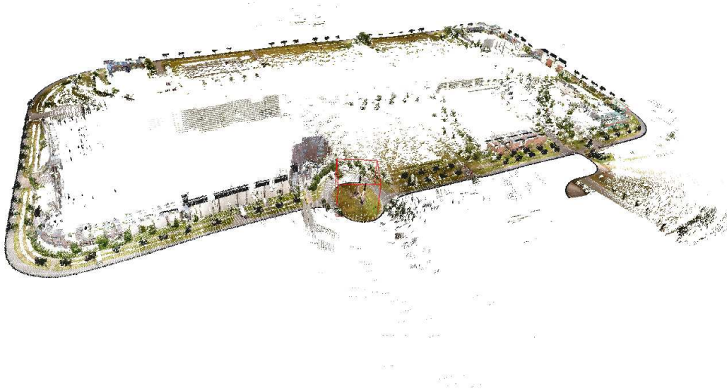
FIGURE 4.9 – 3D representation of 3D laser data and color
