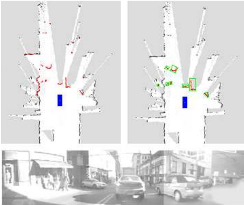
FIGURE 3.9 – Object detection based on occupancy grid.
