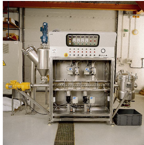
Figure 30: Batch and continuous microwave oven in industry
