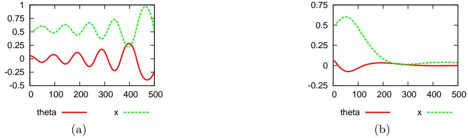
**Fig. 11** Typical behaviors of the position  $x$  of the cart and of the value of  $\vartheta$  for a 100.858 fitness (a) and a 100.965 fitness (b). At  $t = 0$ , the pole starts from  $\vartheta = 0.01$  rad and  $x = 0.5$  m. The controller has to drive the pole to  $\vartheta = 0$  rad and  $x = 0$  m. Controller (a) avoids the pole from falling during this evaluation, but the increasing amplitude suggests an imminent fall.
