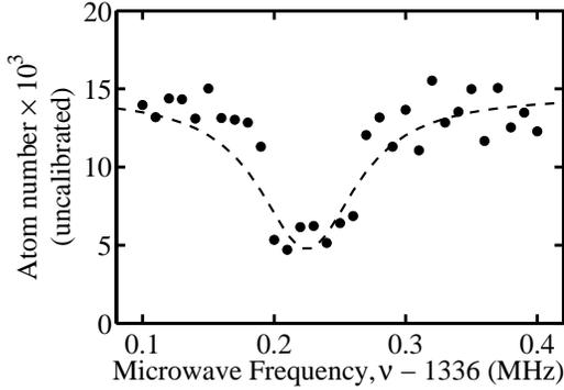
FIGURE 4.13: Microwave transfer in magnetic trap, with 19.8 G Ioffe field. A mixture of atoms in  $|9/2, -9/2\rangle$  and  $|9/2, -7/2\rangle$  is prepared. Shown is a measure of atom number in the  $|9/2, -9/2\rangle$  after microwave sweep. The Lorentzian fit gives the transition centre at  $1336.228 \pm 0.003$  MHz and width of  $0.09 \pm 0.01$  MHz.
