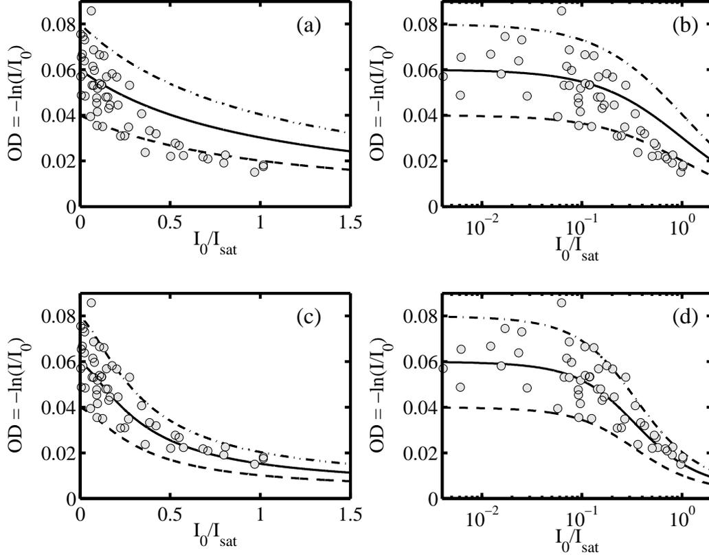
FIGURE B.1: Optical density intensity dependence. Measured optical density OD vs. normalized intensity,  $I_0/I_{\text{sat}}$ . Data is identical in all plots, theory lines neglect Doppler shift, as in from Eq. for (a) and (b); theory lines include Doppler shift for (c) and (d). Theory lines are for  $OD_0 = 0.08$  (dash-dot), 0.06 (solid) and 0.04 (dashed). Left plots are on a linear scale, right plots have a logarithmic  $I_0/I_{\text{sat}}$  scale.
