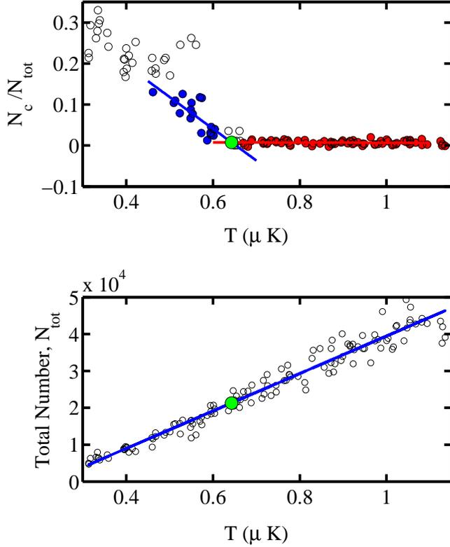
FIGURE C.2: Number calibration using BEC transition temperature. Top: Condensate fraction vs. temperature. Linear fits to the coloured points (red above  $T_C$ , blue below) cross at  $T_C$ . Large green point indicates the location of the crossing of the fits,  $T_C = 640 \pm 40$  nK. Bottom: Atom number as a function of temperature (due to evaporation). Large green point indicates  $T_C$ , where  $N = 21000 \pm 3000$  atoms.
