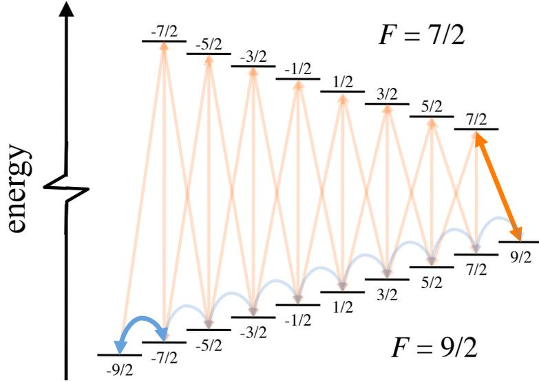
FIGURE 4.11: Ground state manifold of  $^{40}\text{K}$ , in a magnetic field. Lower manifold corresponds to the  $F = 9/2$  hyperfine states; upper manifold corresponds to the  $F = 7/2$  manifold. Small numbers indicate  $m_F$  quantum number, good at low magnetic fields. RF transitions within the hyperfine manifold are schematically shown by blue curved arrows for the lower manifold, while the orange straight arrows correspond to the microwave transitions between hyperfine manifolds.
