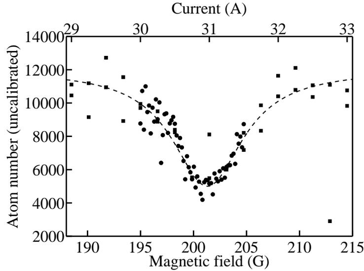
FIGURE 4.14: Experimental evidence of Feshbach resonance in  $^{40}\text{K}$ . Round and square points represent two different data sets, obtained in that order within 1 hour. The magnetic field was calibrated with Zeeman transition frequencies in  $^{87}\text{Rb}$ . The dashed line is a Lorentzian fit to all of the data, with centre at  $201.3 \pm 0.2$  G and width  $8.10 \pm 0.02$  G.
