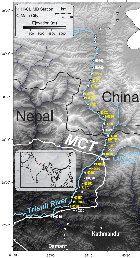
Fig. 4.1: Location of the study area in the Himalayas of Nepal. Inverse white triangles represent the seismological stations from the Hi-CLIMB experiment. Station names are indicated in yellow for stations that are actually used in the Hi-CLIMB dataset and in white when we include all possible sites in the synthetic dataset. MCT refers to Main Central Thrust.
