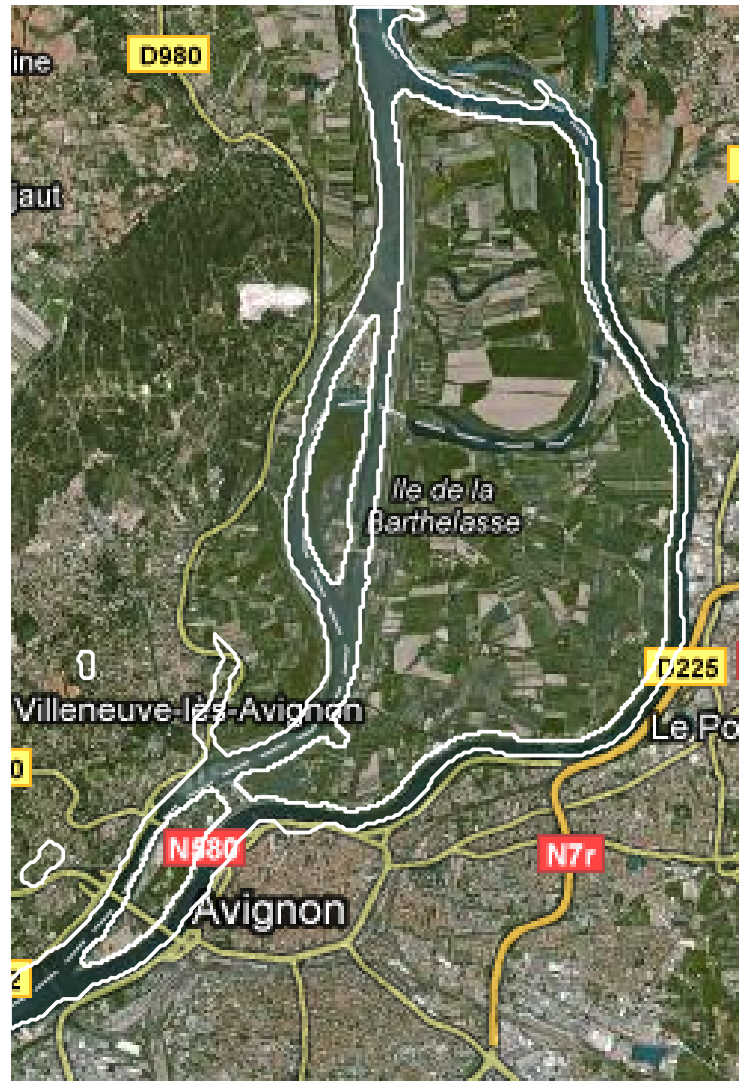
Figure 6.19: Hydrographic network segmentation from a colour image using the directed network model. Flow conservation is satisfied at junctions, illustrated by a significant change of width, and along branches, as illustrated by a slow change of width. ((©2010 Google - Imagery ©2010 TerraMetrics, Map data ©2010 Tele Atlas.)
