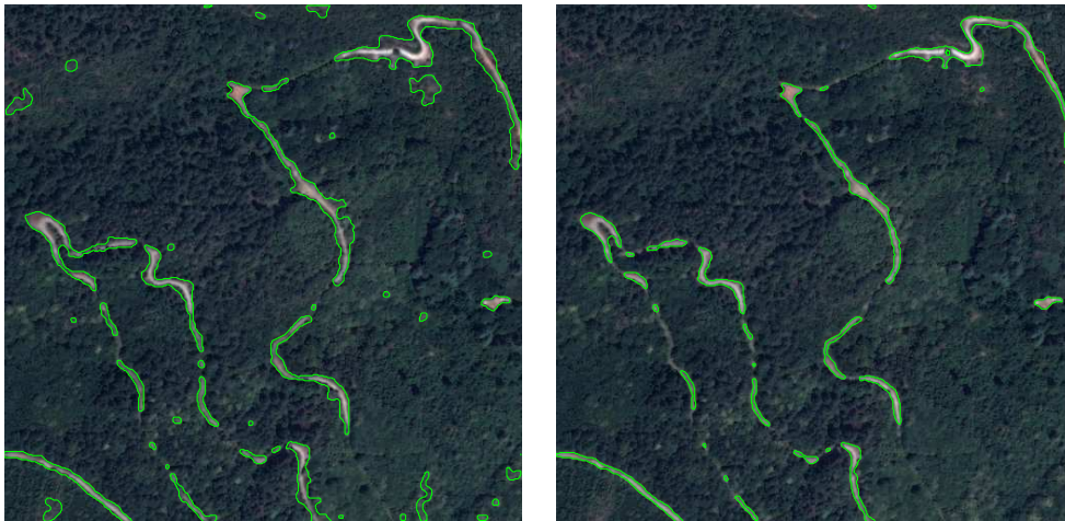
Figure 3.6: Left: segmentation result using parameter values selected from the maroon zone, (w_0, \hat{\alpha}, \lambda_C) = (4, 0.2013, 5) . Right: segmentation result using parameter values leading to an inflection point at the desired bar width, (w_0, \hat{\alpha}, \lambda_C) = (2, 0.7646, 15) .
