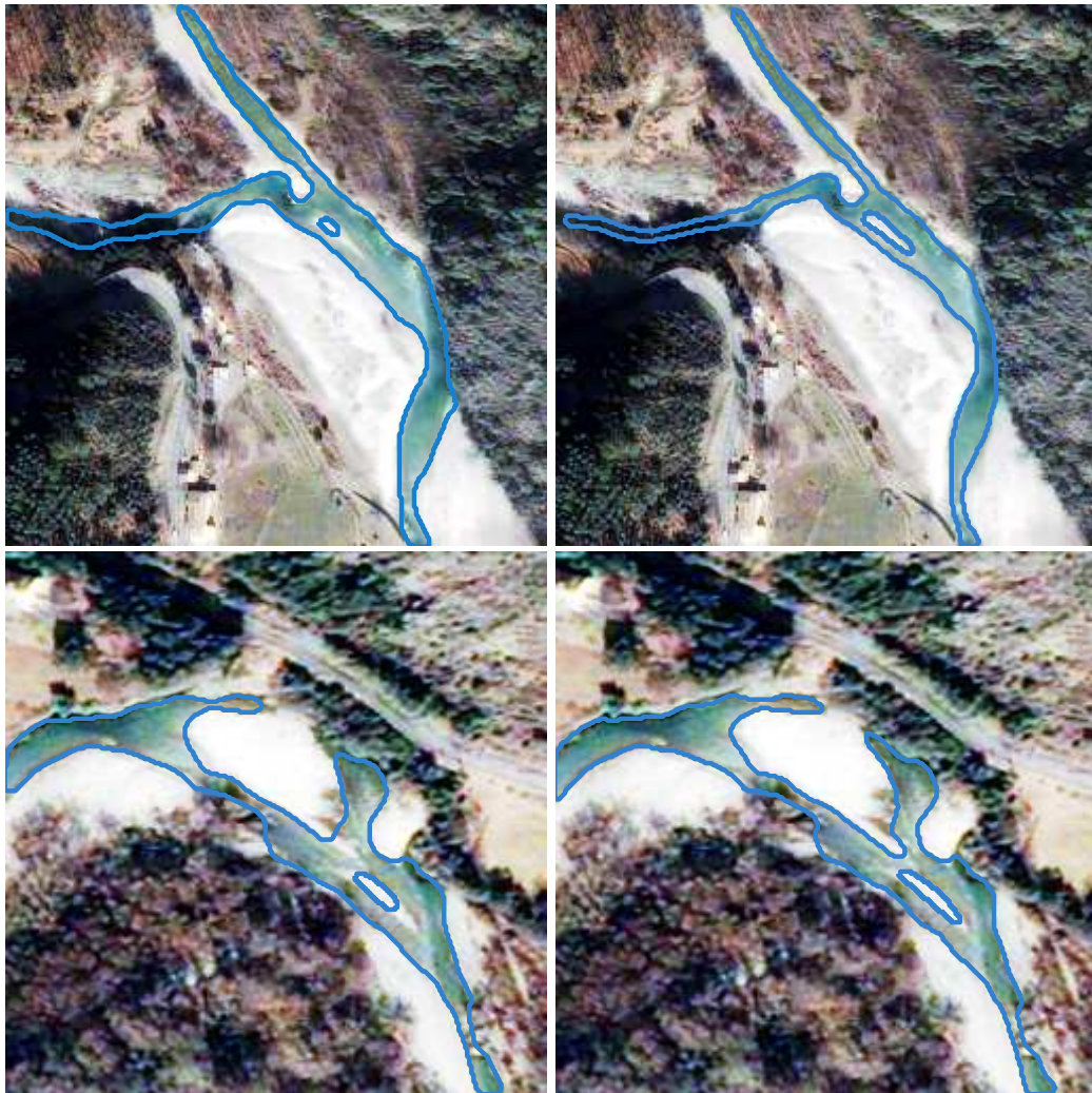
Figure 6.16: Hydrographic network segmentations using the undirected network model (first column) and the directed network model (second column). Regions are obtained by thresholding \phi at 0.
