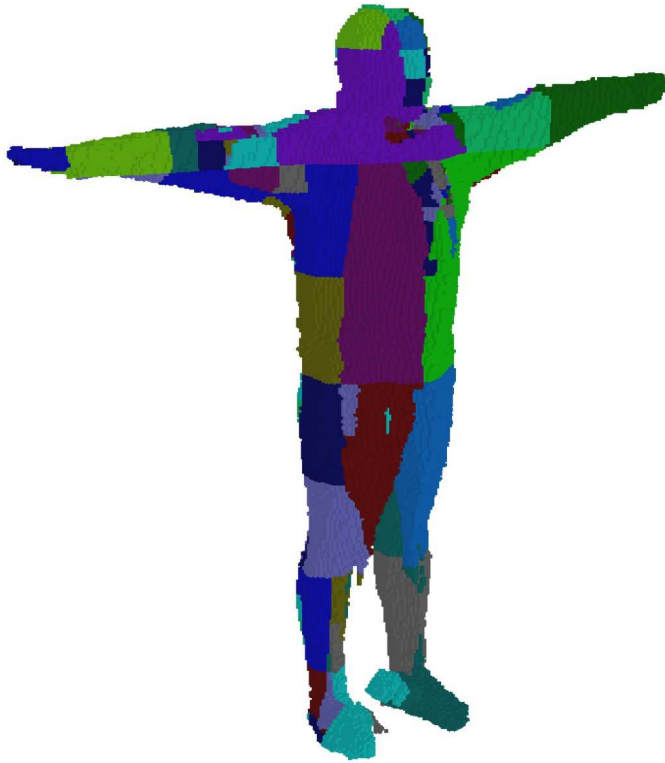
Figure 7.3: Parallel octree carving with 16 cores (max depth of 8). Voxels are color-coded according to the core that produced them. It shows the good spatial locality of work stealing.
