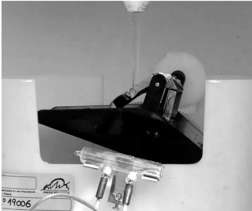
Figure 1: Detail of a tipping-bucket mechanism for rainfall measurement. As it can be seen in a standard recording rain gauge, a small device deployed above the bucket is designed to drive the water flow beyond the barycenter of the system, helping the filled bucket to rock.
