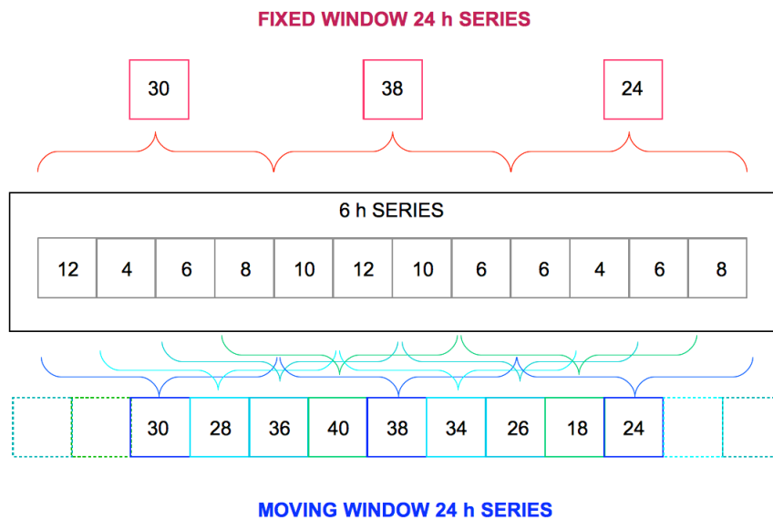
Figure 2.2: Illustration of the fixed-window and moving-window sampling technique for obtaining 24-h data starting from a 6-h database.
