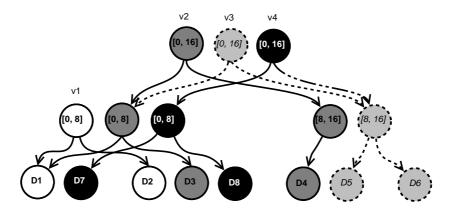
Figure 6.5: Metadata forward references for segment trees: the light-gray segment tree (dotted pattern) has not been generated yet, thus the reference of the black root to its right child (semi-dotted pattern) is a forward reference
