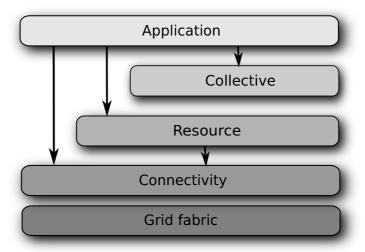
Figure 2.1: Generic architecture of the grid
