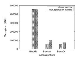
Figure 10.10: Bonnie++ sustained throughput: read, write and overwrite in blocks of 8K (BlockR/BlockW/BlockO)
