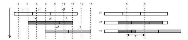
Figure 5.3: Three successive writes (left) and the corresponding snapshots (right)
