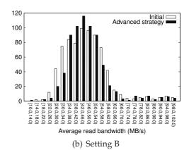
Figure 11.3: Read bandwidth stability: distribution comparison
