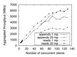
(a) Clients and data providers deployed on distinct physical nodes: throughput improvement under concurrency when increasing the number of available metadata providers
