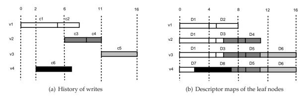
Figure 6.4: Four writes/appends (left) and the corresponding composition of the leaves when lsize = 4 (right)
