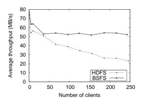
Figure 9.2: Performance of HDFS and BSFS when concurrent clients read from a single file
