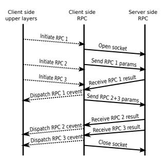
Figure 7.3: RPC layer optimizations: socket reusal, request buffering and aggregation
