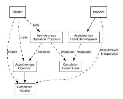
Figure 7.1: Implementing event-driven programming: the proactor pattern
