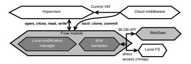
Figure 10.2: Implementation details: zoom on the FUSE module
