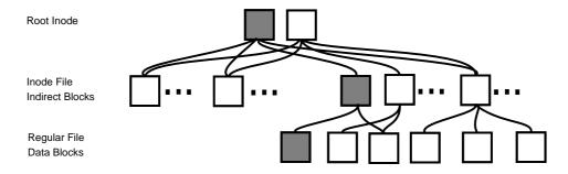
Figure 6.1: Shadowing: updates propagate to the root inode
