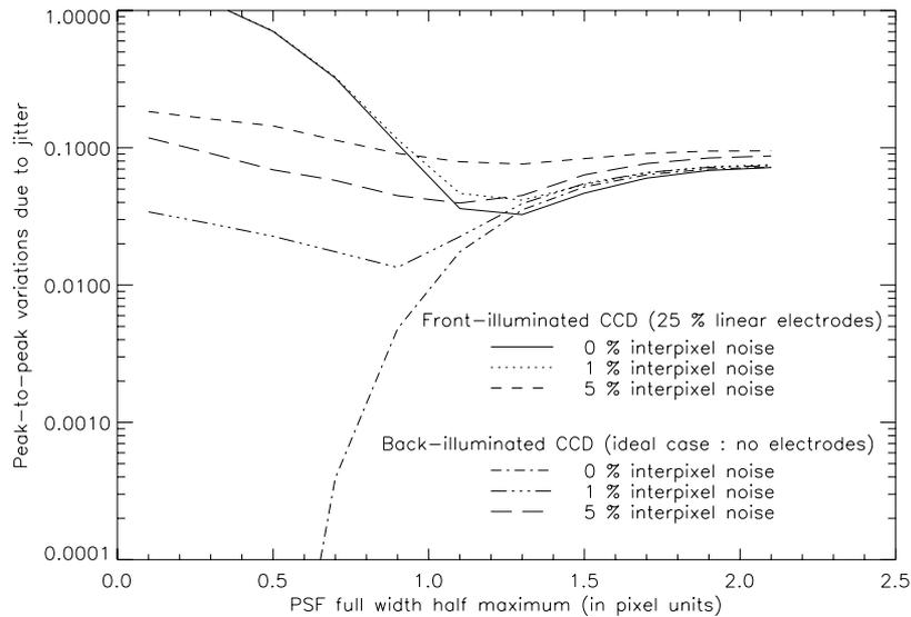
**Fig. 3** Noise as a function of the PSF full width half maximum, for a  $3 \times 3$  pixels photometric aperture. A front illuminated camera (with electrodes), and a back-illuminated camera (as an ideal case with no electrodes) are represented. Three values of interpixel variations are used.
