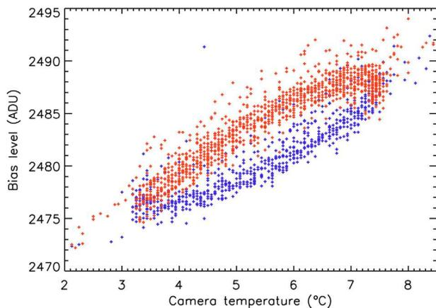
**Fig. 11.** Bias level against the camera temperature for July 11. The blue points correspond to an increasing temperature and the red points to a decreasing temperature, showing a hysteresis behavior.
