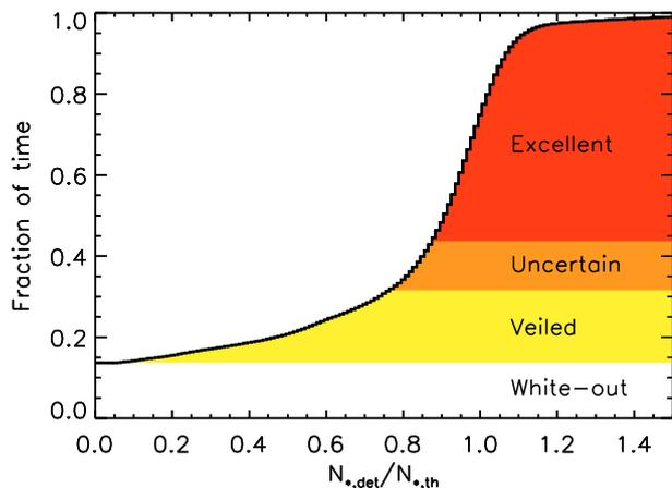
**Fig. 14.** Cumulative histogram of the ratio between the measured and the expected number of stars. The data are distributed between excellent, uncertain and veiled weather. The white part is the fraction of time during which the acquisitions were stopped because of very bad weather (white-out).
