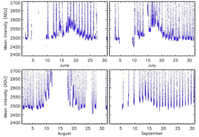
**Fig. 6.** Image intensity. The bias level is around 2480 ADU and the scale is 1% of the CCD dynamics. The sky background increases during 10 days around the full Moon up to typically  $18.1 \text{ mag/arcsec}^2$ .
