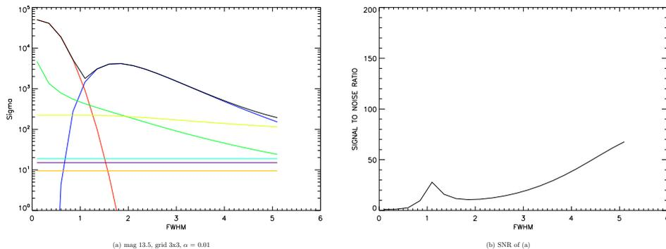
Figure 7: Total noise and signal to noise ratio as a function of the PSF full width half maximum, for a small integration grid (3x3 pixels).
