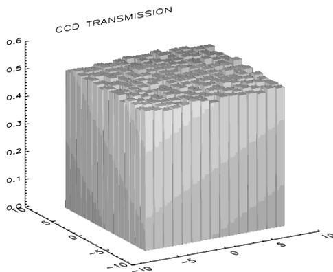
**Fig. 1** Example of the CCD transmission matrix of a front-illuminated camera. The interpixel variations are typically a few per cent. The electrodes cover a part of a pixel and their transmission is very low.
