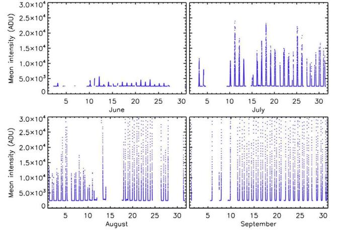
**Fig. 3.** Image intensity for all the winter. The bias level is around 2480 ADU and the scale is half of the CCD dynamics. Peaks around noon will affect the photometry.
