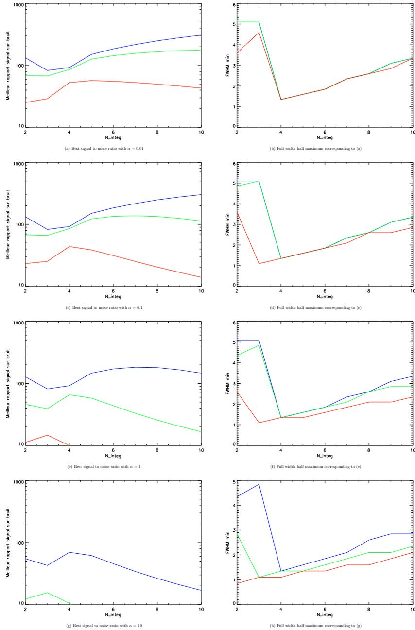
Figure 8: Best signal to noise ratio and corresponding full width half maximum as a function of the integration grid size ( $N \times N$  pixels). Blue curves represent a 11 magnitude star, green curves a 13.5 magnitude star and red curves a 16 magnitude star. Different crowdings are shown, from top to bottom :  $\alpha = 0.01, 0.1, 1$  and  $10$ .
