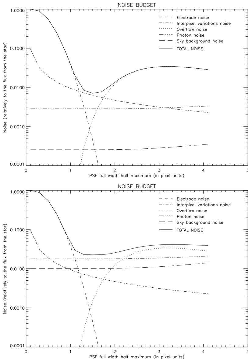
**Fig. 2** Noise budget as a function of the PSF full width half maximum, in a semi-analytical model, for a front illuminated camera with a  $5 \times 5$  pixels photometric aperture and 1% interpixel variations. The results for stars of magnitude 11 (*top*) and 15 (*bottom*) are represented. The CCD dark current and read-out noise are not plotted, and are always lower than the sky background noise.
