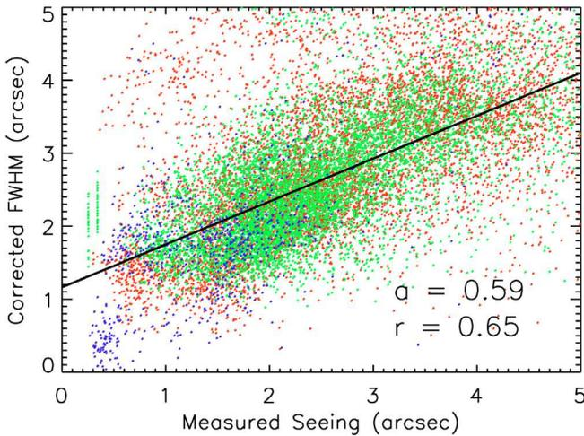
**Fig. 8.** Correlation between the PSF *FWHM* and independent seeing measurements at Dome C, for timescales smaller than one day (the *FWHM* is corrected for larger timescale variations). Direct seeing measurements from three differential image motion monitors are shown in blue, green and red. A linear regression gives a slope  $a = 0.59$  with a correlation coefficient  $r = 0.65$ . The PSFs are clearly affected by seeing variations at the ground level.
