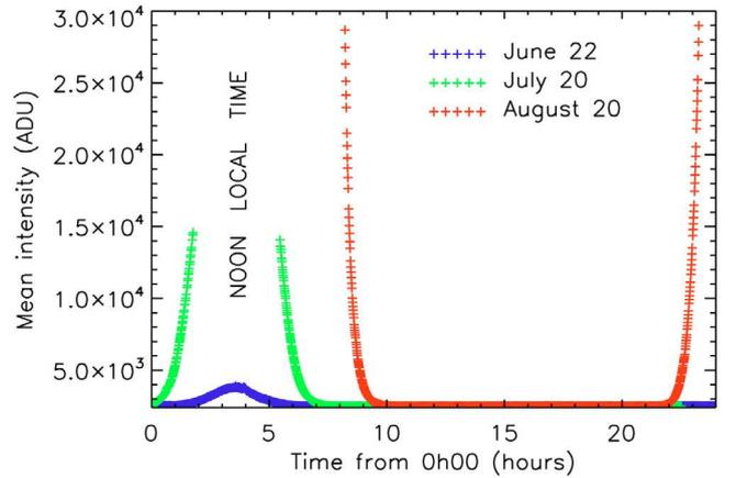
**Fig. 4.** Image intensity during 3 typical days in June, July and August. The bias level is around 2480 ADU and the scale is half of the CCD dynamics. Due to the Sun, the sky background increases around noon. The corresponding magnitude for June 22 is  $15.3 \text{ mag/arcsec}^2$ .
