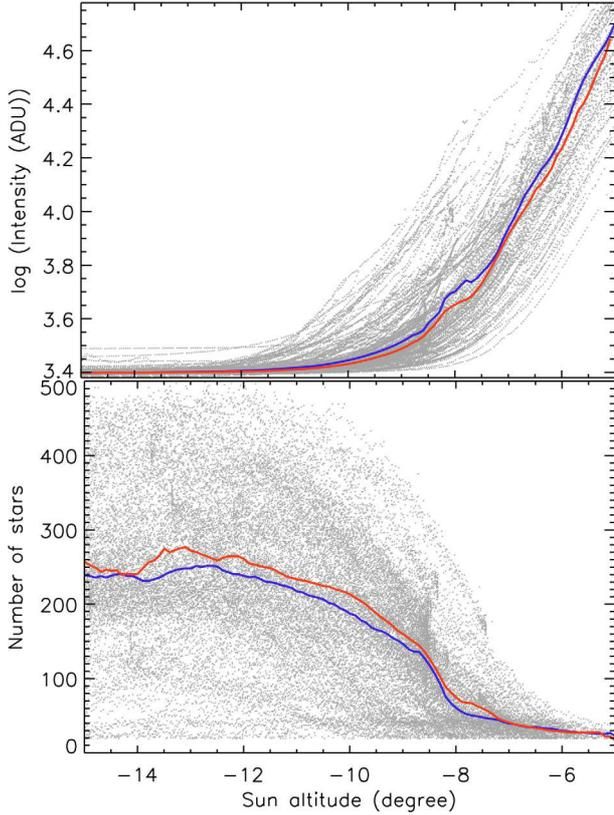
**Fig. 5.** Mean intensity of each image and number of stars as a function of the Sun altitude when it is between  $-15^\circ$  and  $-5^\circ$ . The bias level is around 2480 ADU and the intensity scale is the whole CCD dynamics. Points: individual measurements, blue and red: average during ascending and descending periods respectively. At  $9^\circ$  below the horizon the sky brightness is  $16.6 \text{ mag/arcsec}^2$ .
