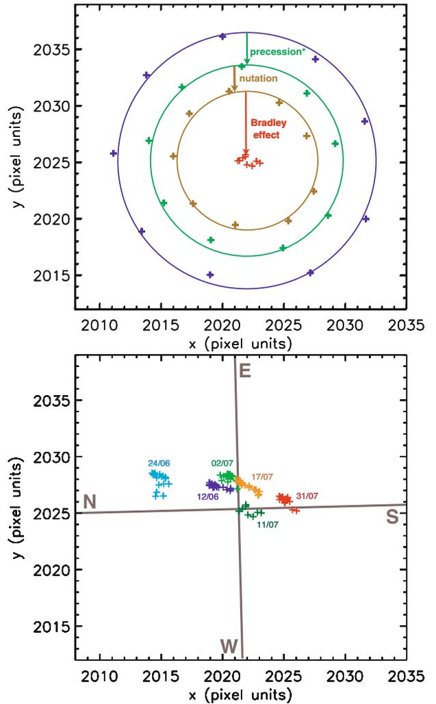
**Fig. 9.** Position of the pole on the CCD. *Top*: 9 images on July 11 after various astrometric corrections (blue: approximate correction of the precession of the equinox, green: improved correction of the precession of the equinox, brown: correction of the nutation, red: correction of the Bradley effect). *Bottom*: 7 days between June 12 and July 30, showing a drift over the winter (dark blue: June 12, light blue: June 24, green: July 2, yellow: July 11, orange: July 17, red: July 30).
