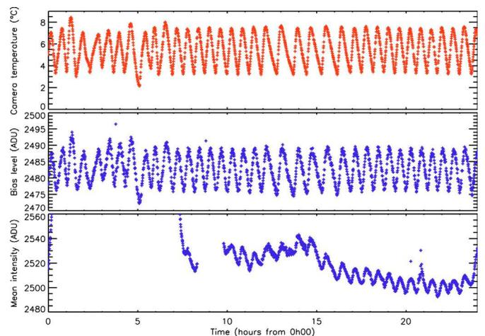
**Fig. 10.** Camera temperature, bias level and image intensity on July 11. The camera temperature varies between  $+4$  and  $+8\text{ }^{\circ}\text{C}$  with a period of one hour and affects the bias level and the image intensity to about 10 ADU.
