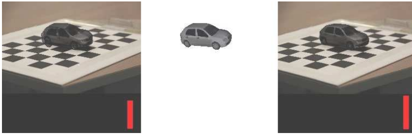
Figure 5.16: Initial pose (left two images) and result of the registration after convergence (right two images) using the best-scoring 3D car model for one image of the test sequence. The first columns show the test images with the 3D model in the current pose overlaid; the red bar indicates the similarity score.
