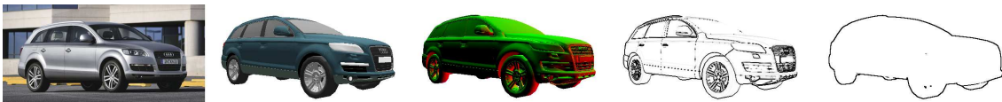
Figure 2.7: Real object (left) and some outputs generated from its corresponding 3D CAD model (left to right: intensity, surface normals, color gradients, surface contour).
