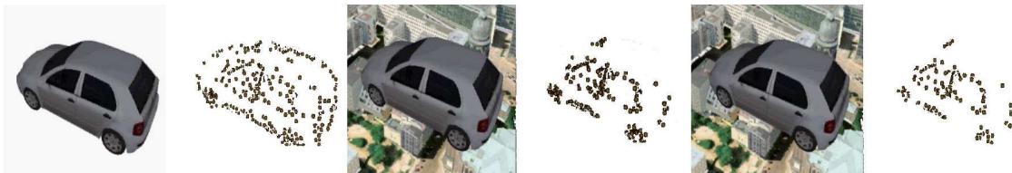
Figure 3.4: Different steps of discriminative filtering for one pose: initial features (left), intermediate step (center), final result (right).
