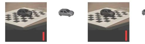
Figure 5.16: Initial pose (left two images) and result of the registration after convergence (right two images) using the best-scoring 3D car model for one image of the test sequence. The first columns show the test images with the 3D model in the current pose overlaid; the red bar indicates the similarity score.
