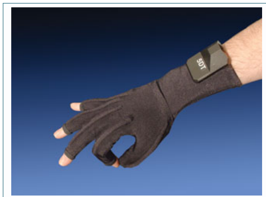
Figure 46: Le Data Glove Ultra de Fifth Dimension Technologies .
