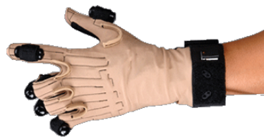
Figure 49: Le gant CyberTouch de Cyber Gloves Systems .
