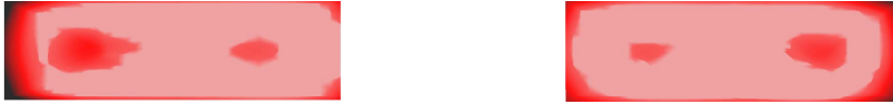
Figure 3.22: Current displacement in the conductor cross section of the two turn side of the test inductor. Plot obtained by HFSS-simulation of the test-inductor, current density in logarithmic scale increasing to darker colors (see figure 3.23). The slightly higher current in the very inside of the metal is due to simulation artifacts.
