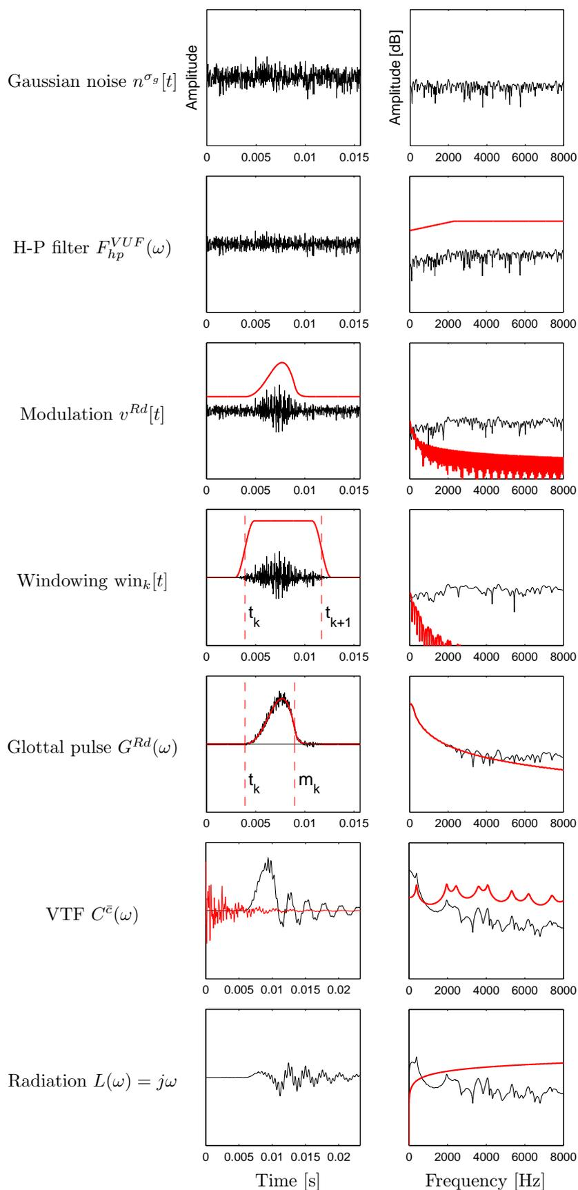
Figure 9.2: Synthesis of a segment (For the clarity of this sequence of plots, the difference of level between the deterministic and random components may not correspond to the descriptions given by the text)
