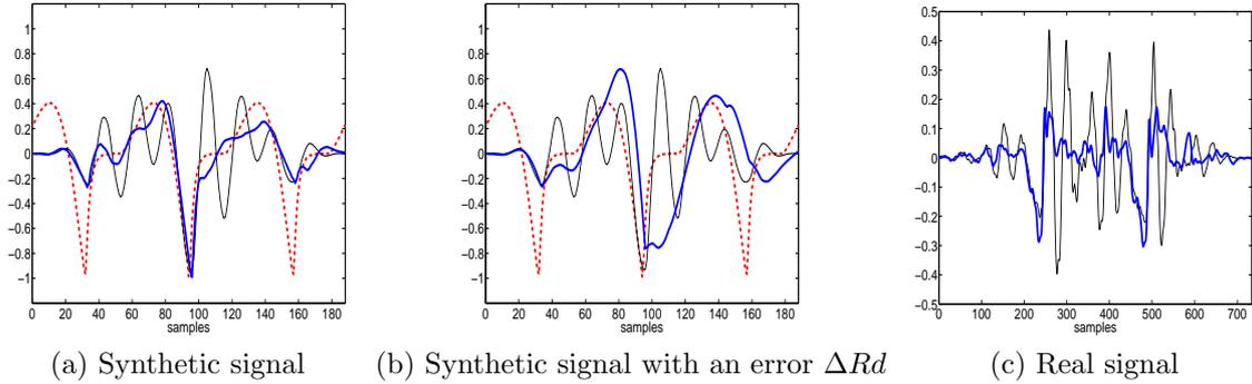
Figure 7.1: Examples of radiated glottal source  $\tilde{G}'(\omega)$  in the time domain: (a,b) Synthetic signals using the  $LF^{Rd}$  glottal model with  $f_0 = 128$  Hz  $Rd = 1$  and a /e/: the waveform in thin black line, the synthetic source in dashed red line and  $\tilde{G}'(\omega)$  in thick blue line. (c) Real signals: the waveform in thin black line and  $\tilde{G}'(\omega)$  in thick blue line.
