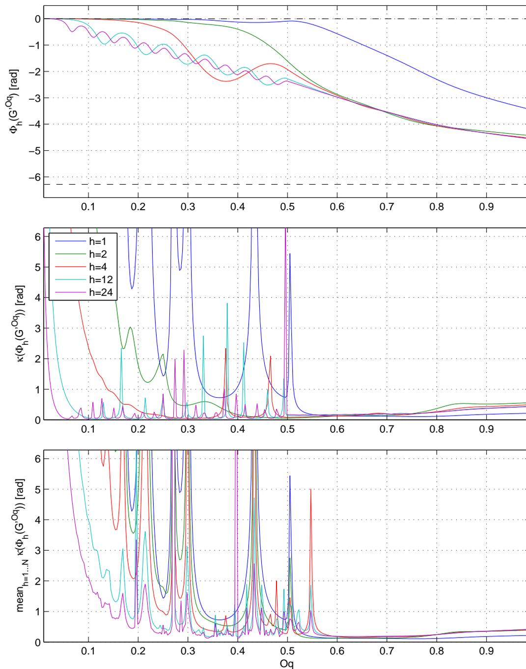
Figure 6.7: FPD  $\Phi_h$ , conditioning measure  $\kappa$  and mean conditioning measure for the Rosenberg <sup>$O_q$</sup>  glottal model.
