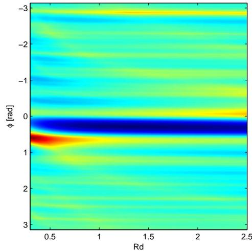
Figure 5.1: Example of  $\text{MSP}(Rd, \phi, 12)$  computed on a synthetic signal. The colder the color, the smaller the mean squared phase. The optimal parameters are  $Rd \approx 1.5$  and  $\phi \approx 0.3$ .
