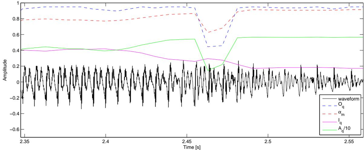
Figure 5.7: The parameters  $(I_q, A_q)$  from the estimation of  $(O_q, \alpha_m)$  using MSP on a real speech segment. The waveform in plain black line and the parameters in color according to the legend. One can see that  $O_q$  and  $\alpha_m$  offset each other in order to keep a relatively smooth time evolution of  $I_q$  whereas  $A_q$  represents the underlying irregularities.
