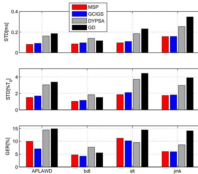
Figure 8.5: Evaluation of GCI estimation methods with 4 databases. STD is the standard-deviation computed through the interquartile range of the duration between the reference and the estimated GCIs, given in milliseconds [ $ms$ ] and in percent of the period [ $\%T_0$ ]. The Gross Error Rate (GER) is the percent of that same durations  $> 0.1 \cdot T_0$  among all comparison pairs.
