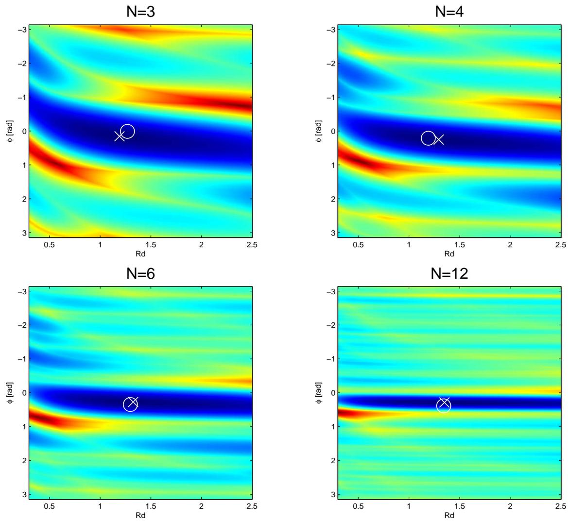
Figure 5.2:  $MSP(Rd, \phi, N)$  surface while increasing  $N$ . The colder the color, the smaller the mean squared phase. Starting values of each step are indicated with a circle and the final steps of Preconditioned Conjugate Gradient are shown with a cross.
