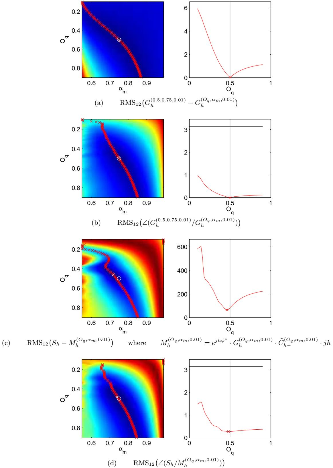
Figure 5.4: RMS of the first 12 harmonics for  $(\alpha_m, O_q)$  using the LF model ( $O_q^* = 0.5, \alpha_m^* = 0.75, Q_a^* = 0.01$ ). The RMS is shown to the left with colors (the colder the color, the smaller the RMS) and to the right by the ordinate. In red line, the right column shows the function of minimum error for each line of the error surface. Horizontal and vertical lines show respectively the optimal value and the maximum error.
