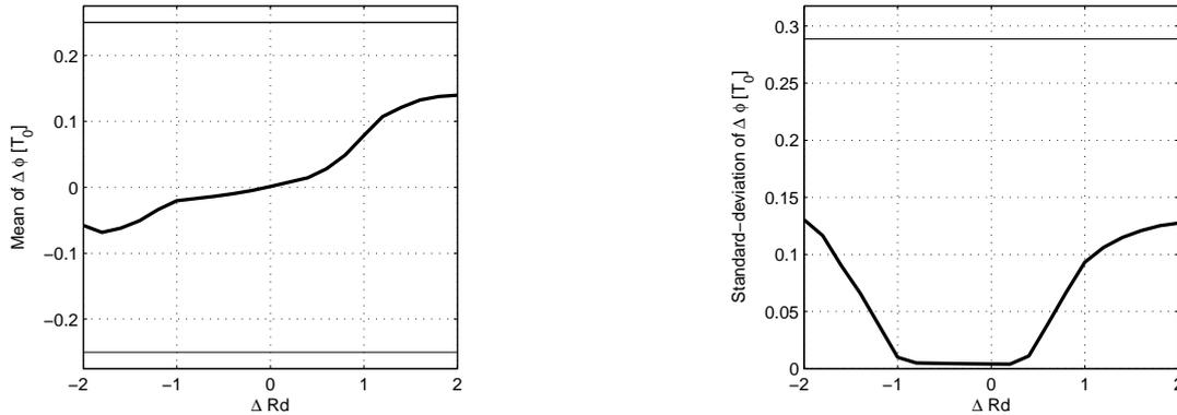
Figure 7.4: In thick line, the error of the GCI estimator related to an error of the shape parameter  $Rd$ . In thin line, the mean estimator (this estimator return a random delay in  $[0.5/f_0; 0.5/f_0]$ ) for the plot of the standard-deviation. For the plot of the mean error, the absolute value of the position error is used  $|t_{GCI} - t_{GCI}^*|$ .
