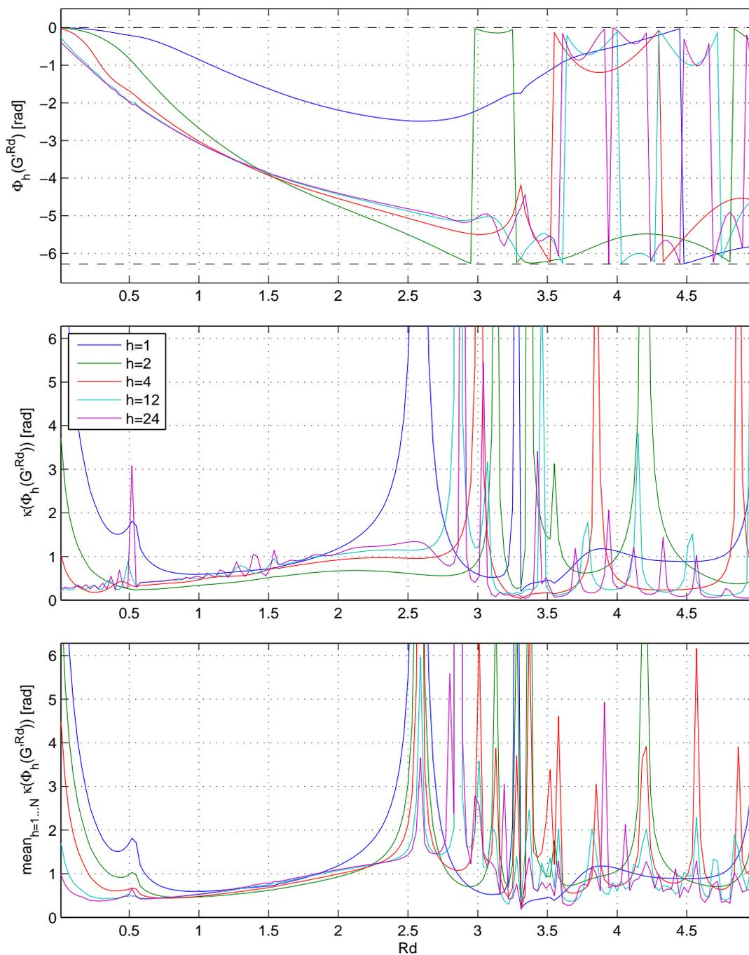
Figure 6.5: For the  $LF^{Rd}$  glottal model: its Functions of Phase Distortion (FPD)  $\Phi_h$  to the top. The conditioning measure  $\kappa$  in the middle and the mean conditioning measure related to the method  $FPD^{-1}$  to the bottom. From the conditioning measures, one can see that the shape parameter can be estimated only in the interval  $[0; 2.5]$ .
