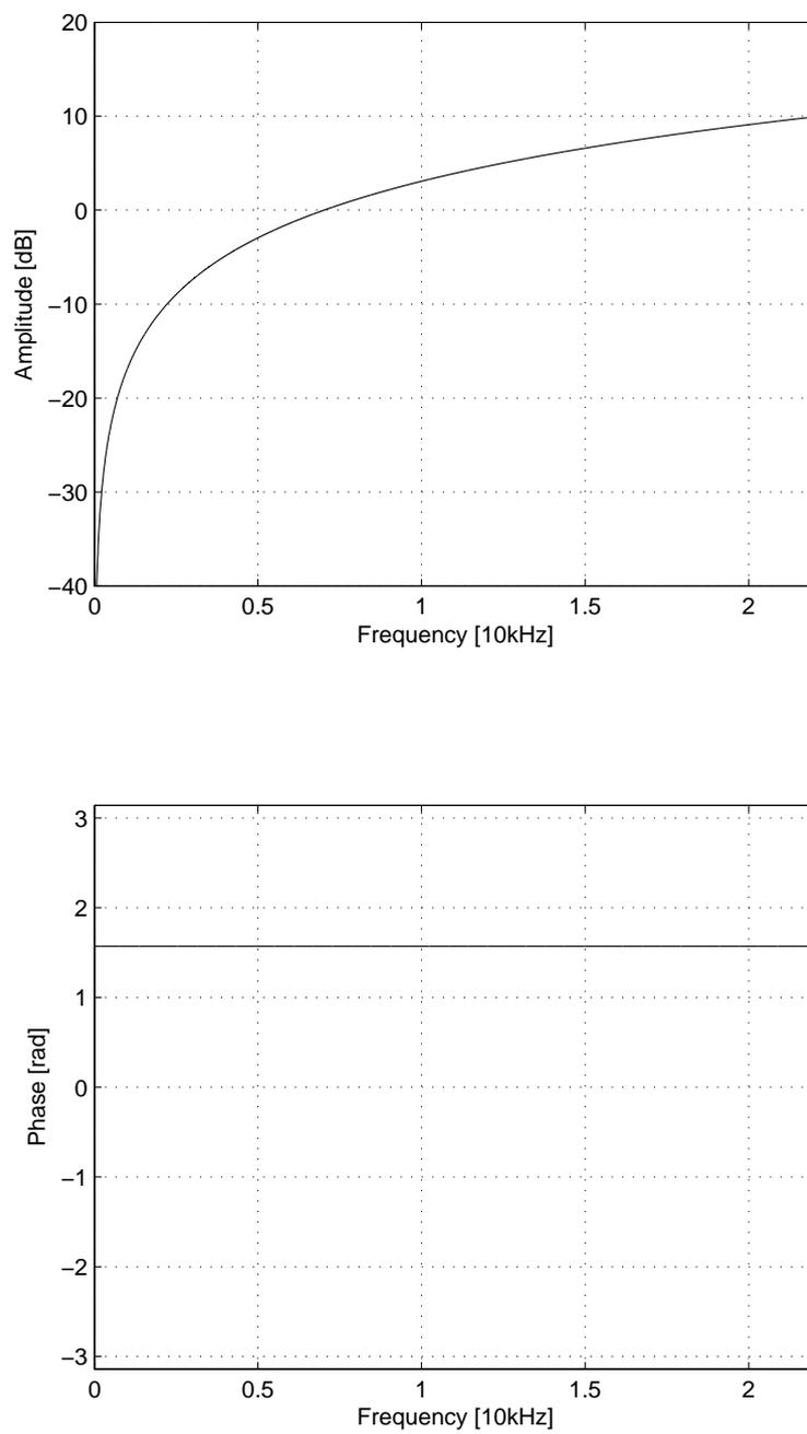
Figure 3.2: The radiation model  $L(\omega) = j\omega$
