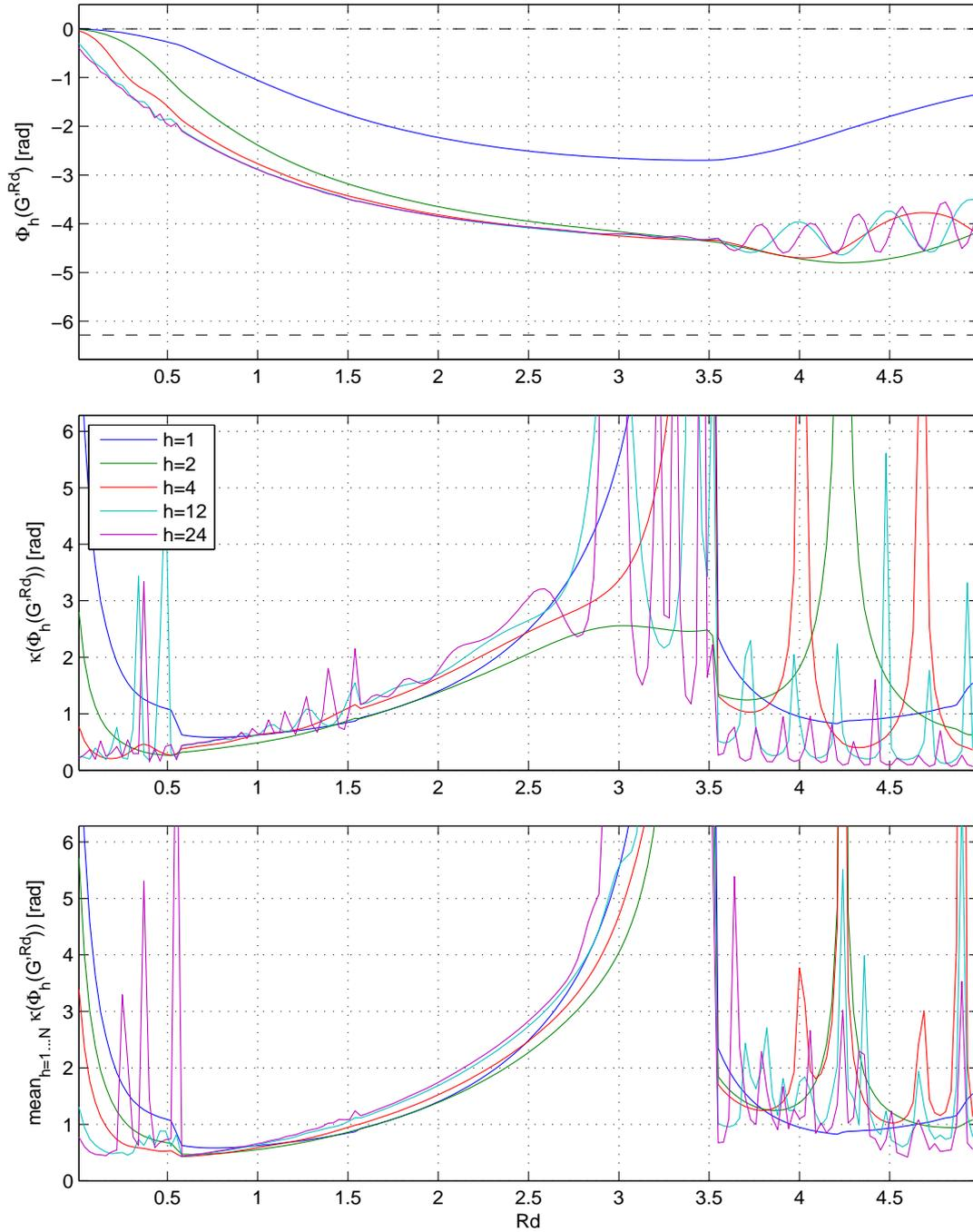
Figure 6.6: FPD  $\Phi_h$ , conditioning measure  $\kappa$  and mean conditioning measure for the CALM<sup>Rd</sup> glottal model.
