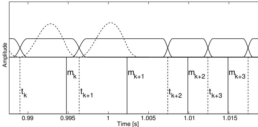
Figure 9.1: Two voiced segments followed by two unvoiced segments: Marks  $m_k$  and starting times  $t_k$  are shown with vertical lines. Synthesized  $\text{LF}^{Rd}$  models are in dashed lines, and windows  $\text{win}_k[t]$  are in solid lines.
