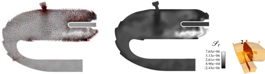
Figure 9.6: Instantaneous view of the heat flux vector field (left) and radiative source term (right) in cut 2
