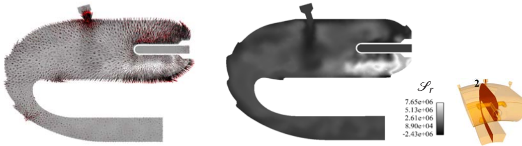
Figure 9.6: Instantaneous view of the heat flux vector field (left) and radiative source term (right) in cut 2
