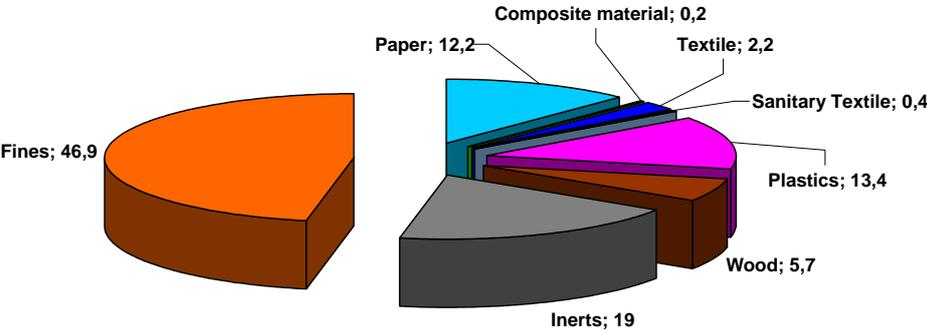
**Figure VI- 47: Percentage composition by dry weight of Drill Sample N6.**
