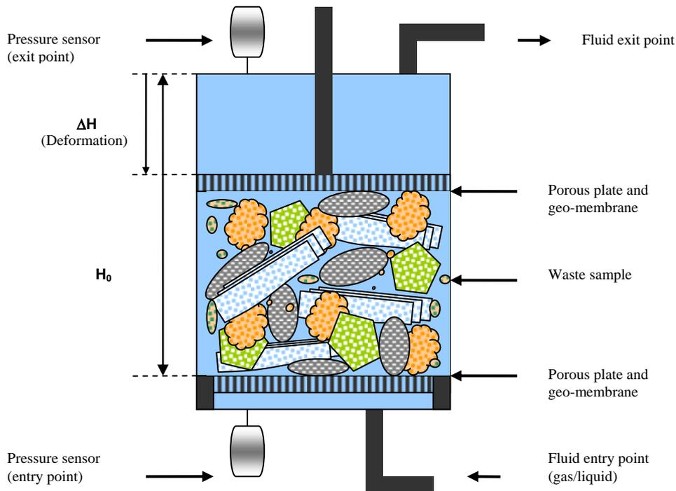
**Figure II- 14: Schematic diagram of the Oedopermeameter.**
