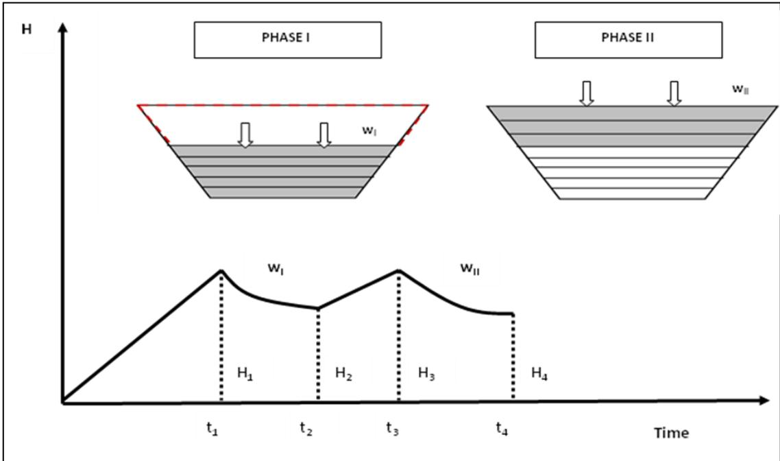
Figure V- 37: Construction of waste column in two phases for Cell 'C' of chatuzange landfill site.
