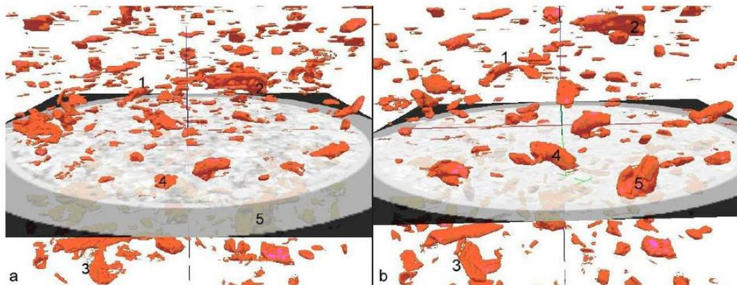
**Figure II- 10: 3D image of reactor 2 showing only objects with CT number between 200 and 900, corresponding to bone and other dense materials. The uniform grey area represents the plane at the centre of the midpoint piezometer port to provide absolute location (Watson, et al., 2007) Figure ‘a’ is related to the scan prior to degradation while ‘b’ shows the scan after 2 months of degradation.**
