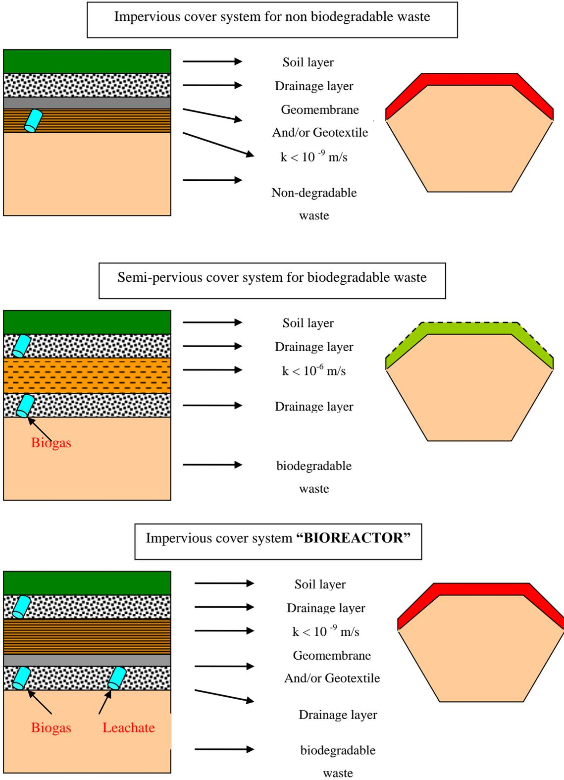
Figure I-15 : Types of cover lining systems in reference with the waste landfilled.
