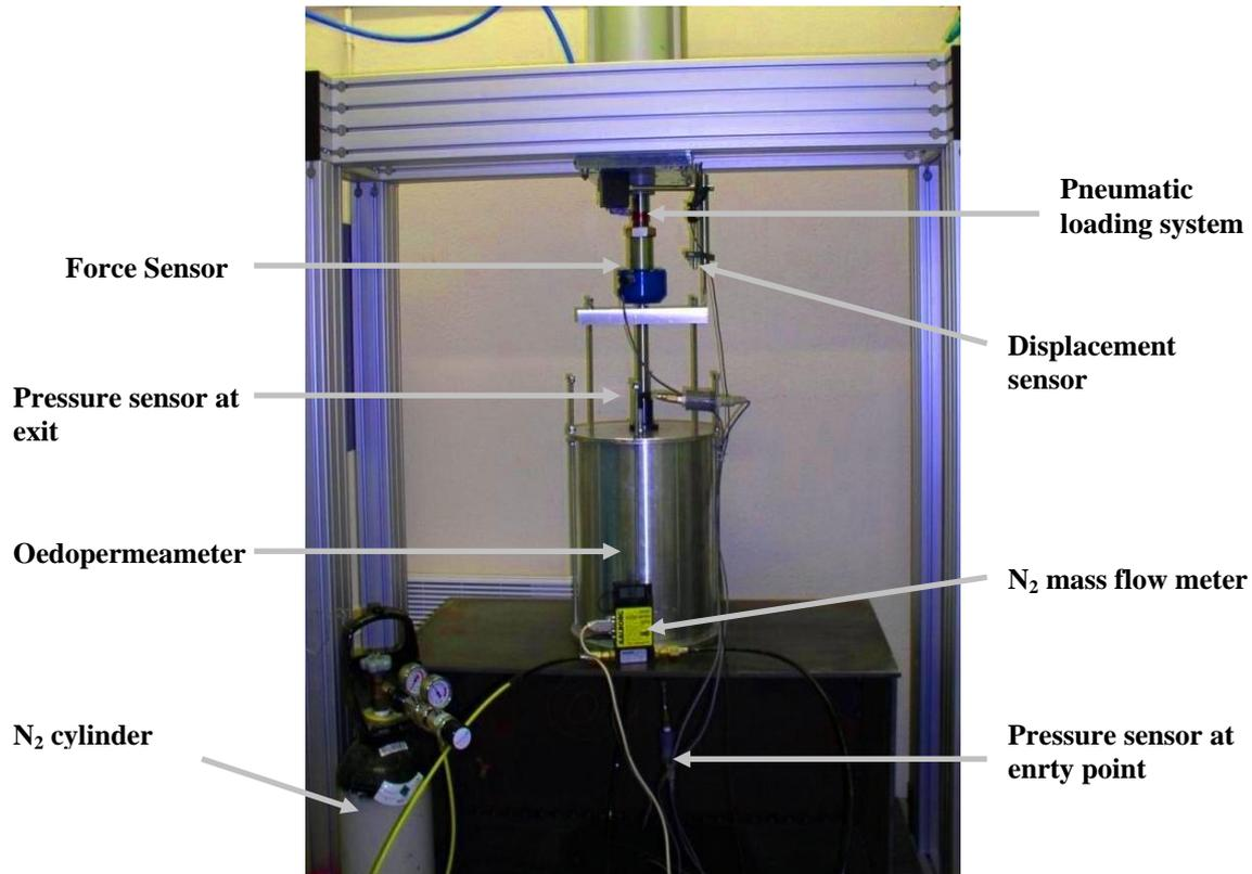
**Figure II- 15: Oedopermeameter connected with complimentary equipment.**
