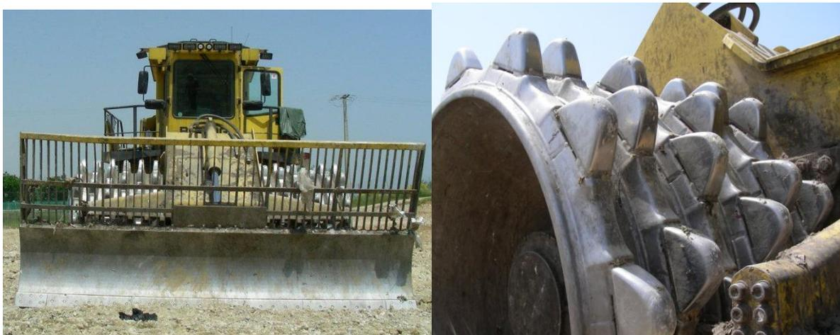
**Figure I-11 : Spreading and compaction vehicle (Sheep foot roller).**
