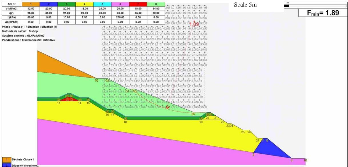
Figure VI- 54: Stability analysis of Case 3 for sample N6 with a calculated factor of safety = 1.89.
