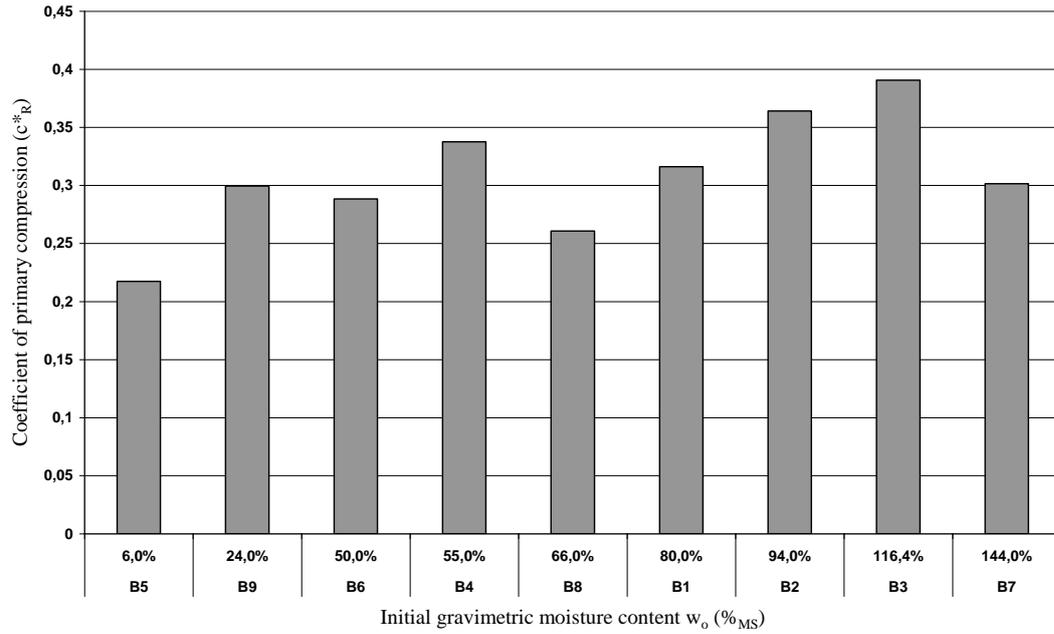
**Graph III- 5: Coefficient of primary compression  $C_R^*$  as a function of initial gravimetric moisture content for the compression-gas permeability experiments carried out in the oedopermeameter (waste ‘B’).**
