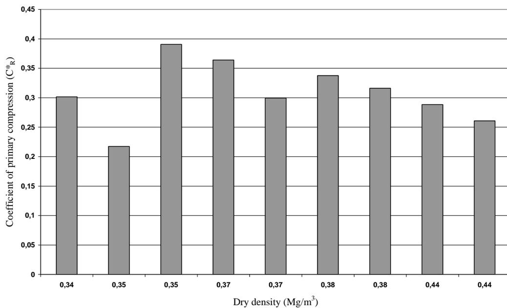
**Graph III- 6: Coefficient of primary compression  $C_R^*$  as a function of initial dry density at the pre-consolidation compression stress of respective waste sample for the compression-gas permeability tests carried out in oedopermeameter cell (Waste ‘B’).**
