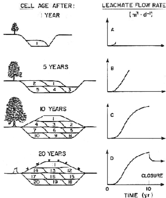
**Figure I-7 : Leachate flow rate for different waste component categories (A, B, C and D) as a function of time (Farquhar, 1989).**
