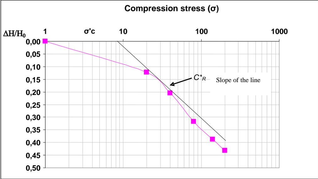
**Figure III- 4: Determination of pre-consolidation stress.**
