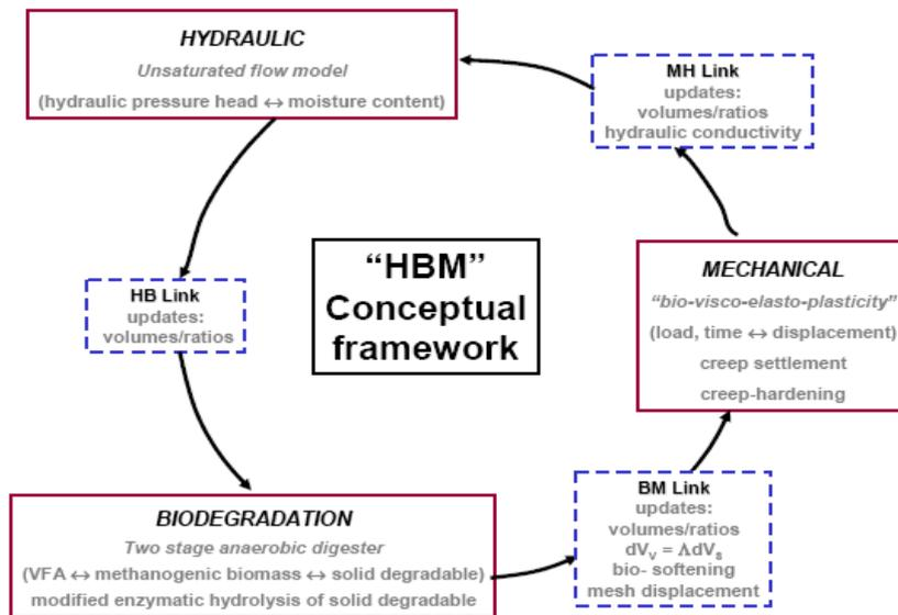
**Figure V- 18: Schematic diagram with the components of the HBM model (McDougall et al., 2005).**
