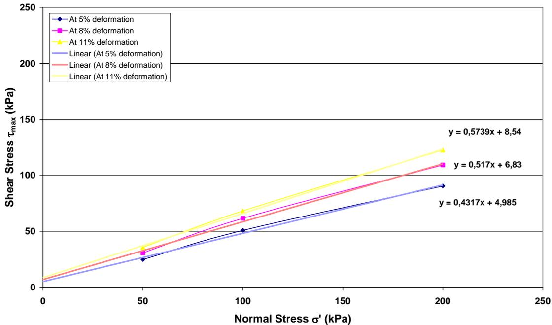
**Figure VI- 29: Determination of shear strength values (cohesion  $c$  and friction angle  $\phi$ ) from the graph of normal stress and shear stress (test sample LMD-0, § VI-3.2.5).**
