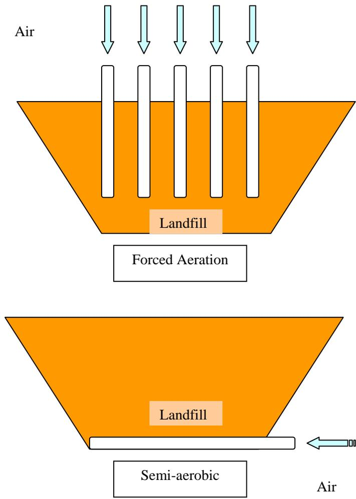
**Figure I-19 : Comparison of two in-situ aeration processes.**
