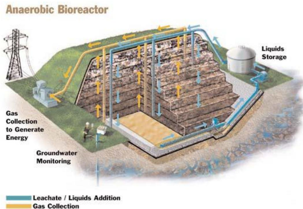
Figure I-21 : Anaerobic Bioreactor (Waste Management, 2000).
