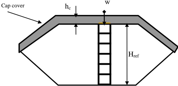
**Figure V- 22: Typical landfill waste column construction.**
