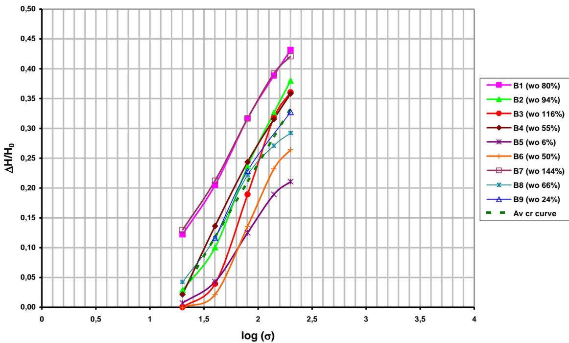
Graph III- 4: Determination of coefficient of primary compression.
