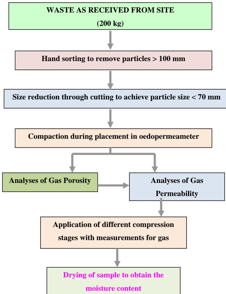
Figure III- 9: Schematic diagram for the oedopermeameter tests.
