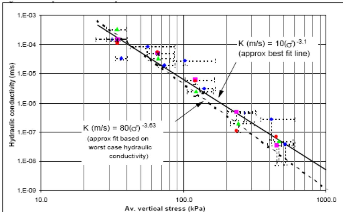
**Figure II- 8: Reduction in hydraulic conductivity with increasing effective stress (Powrie et al., 2000).**
