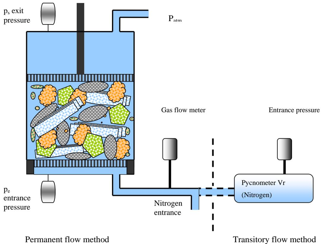
**Figure II- 17: Apparatus arrangement for gas permeability measurement for permanent and transitory flow methods.**
