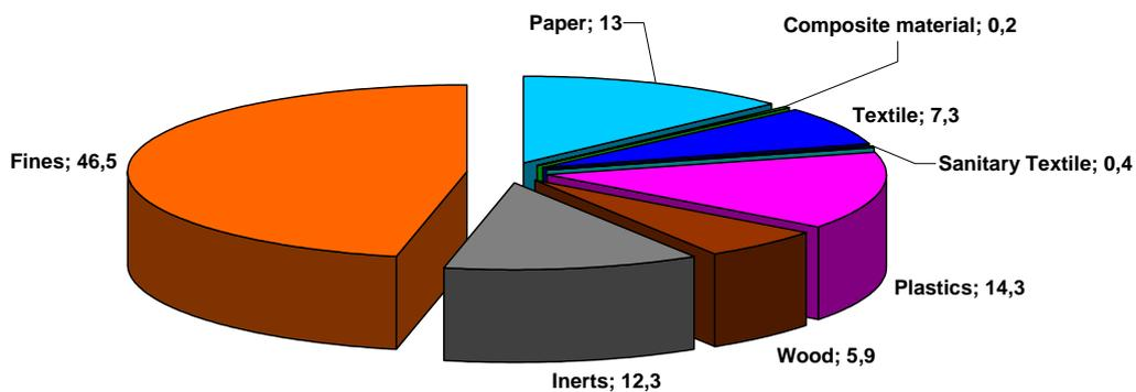
**Figure VI- 44: Composition of Waste of drilled samples N3.**
