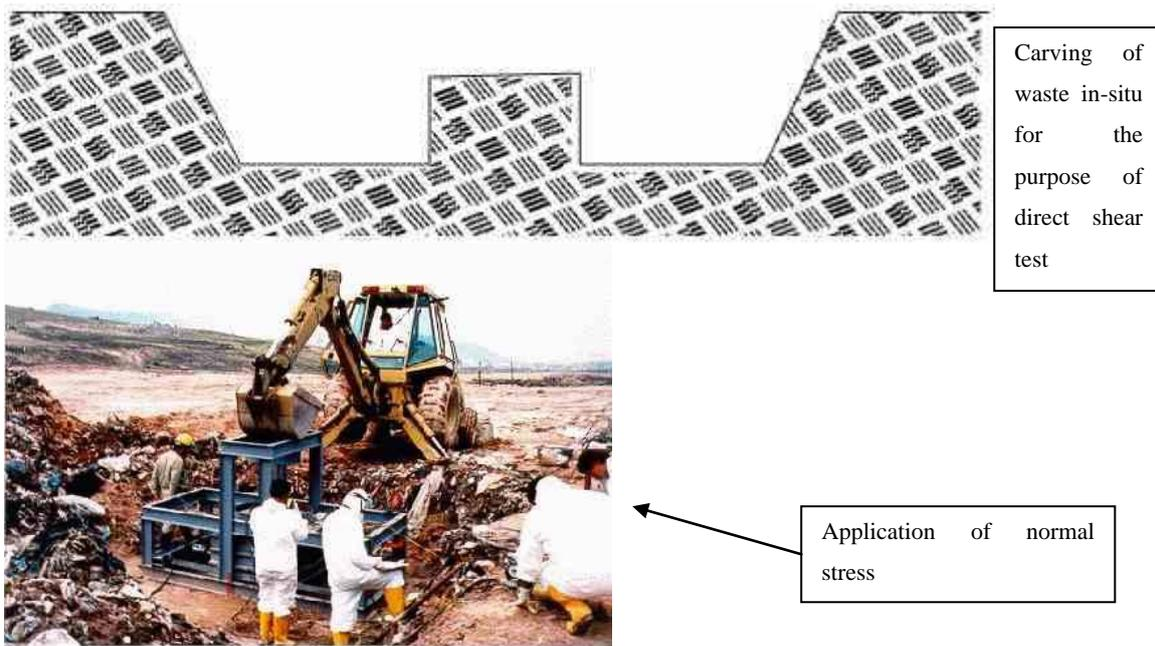
**Figure VI- 22: In-Situ direct shear test. (Caicedo et al., 2007).**
