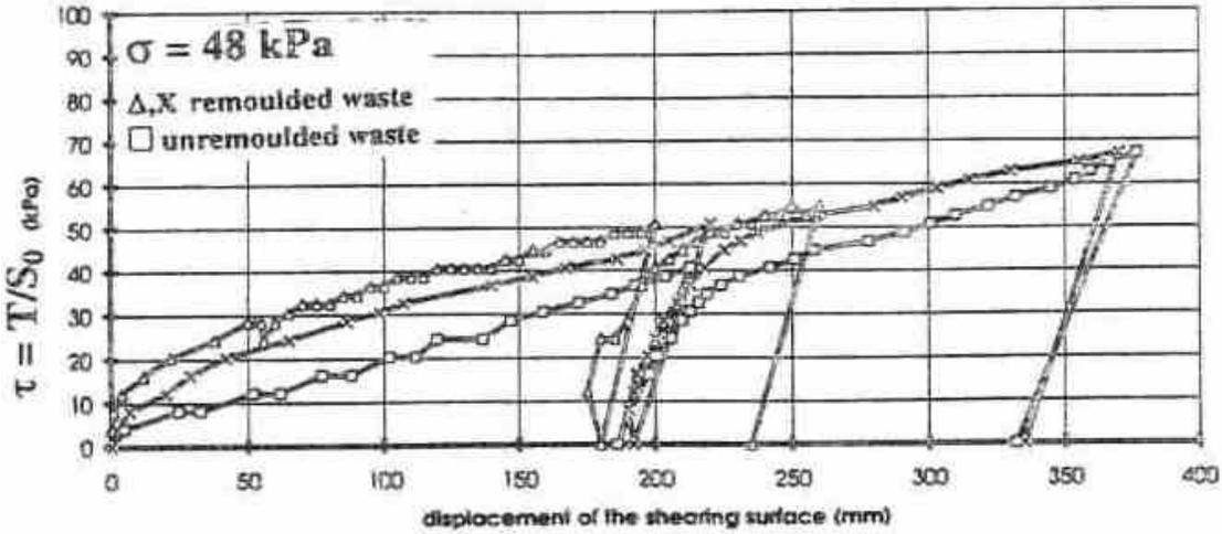
Figure VI- 4: Shear test results (Gotteland et al. 1995).
