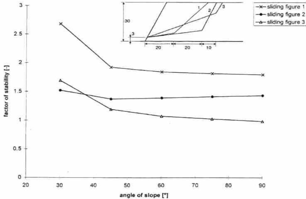
**Figure VI- 8: Slope failure calculations for different sliding figures with material values of fresh waste (Kölsch, 1995).**
