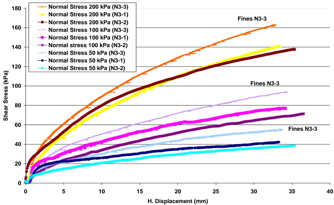
**Graph VI- 11: Comparison of shear strength of samples at initial grain size and composition (N3-1 and N3-2) with the sample after sieving < 20 mm (N3-3) normally consolidated at a displacement rate of 1 mm/min.**
