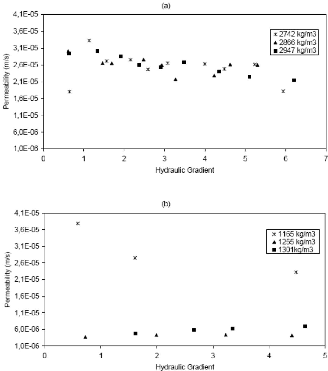
**Figure II- 9: The values of permeability for MSW samples at field capacity (saturated and drained under the effect of gravity) tested under different densities and hydraulic gradients in (a) small-scale device; (b) large-scale device (Durmusoglu et al., 2005).**
