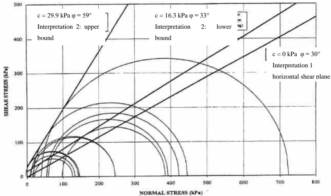
**Figure VI- 18: Mohr-coulomb stress envelope, different approaches (Kavazanjian et al., 1999).**
