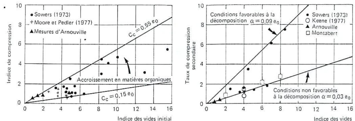
**Figure V- 23: Index of primary ( $C_c$ ) and secondary compression ( $C_\alpha$ ) for domestic waste according to the initial void ratio  $e_0$  – Spindle of Sowers taken again by Cartier and Baldit (1983).**
