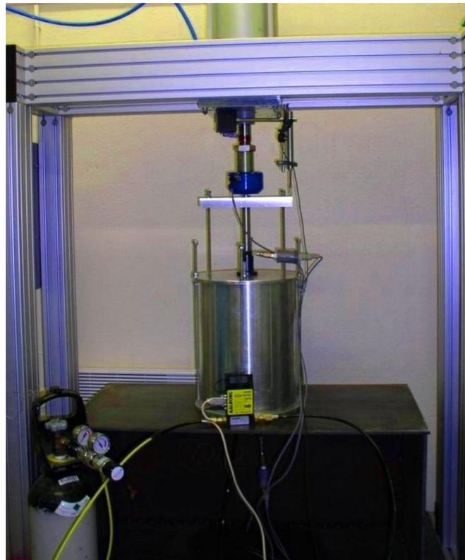
**Figure III- 1: Apparatus arrangement for gas permeability measurement.**
