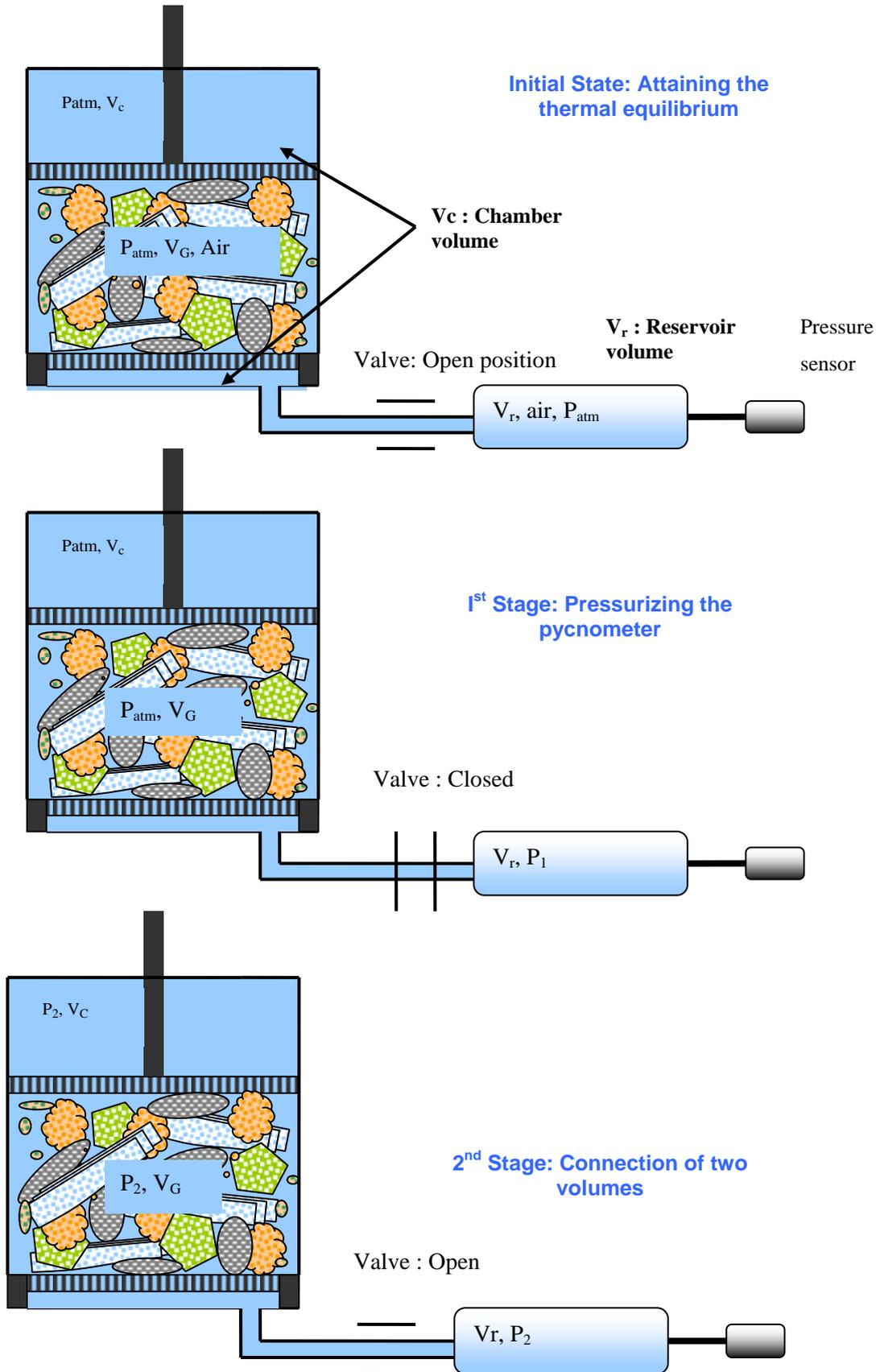
Figure II- 16: Steps for gas porosity measurement.
