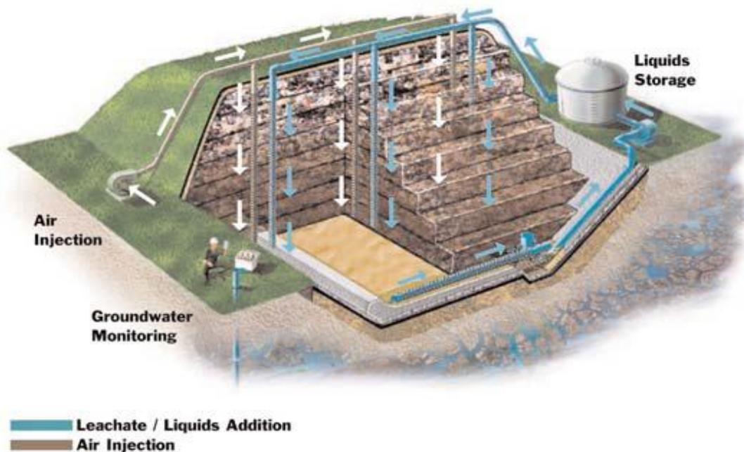
Figure I-23 : Aerobic Bioreactor (Waste Management, 2000).
