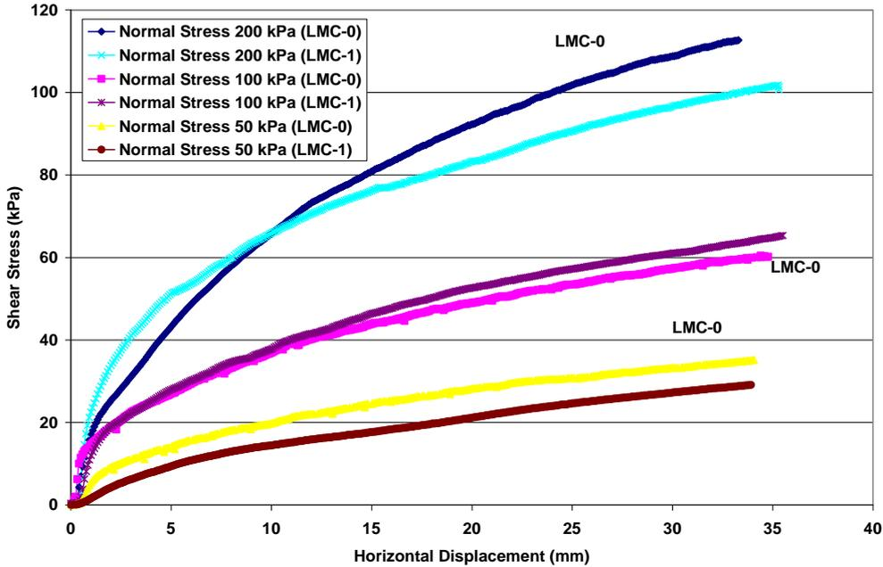
**Graph VI- 7: Comparison of shear behaviour of excavated samples (LMC-0) with the shredded samples (LMC-1).**
