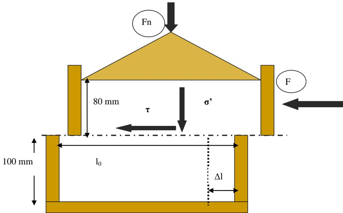
**Figure VI- 26: Schematic diagram of direct shear box.**
