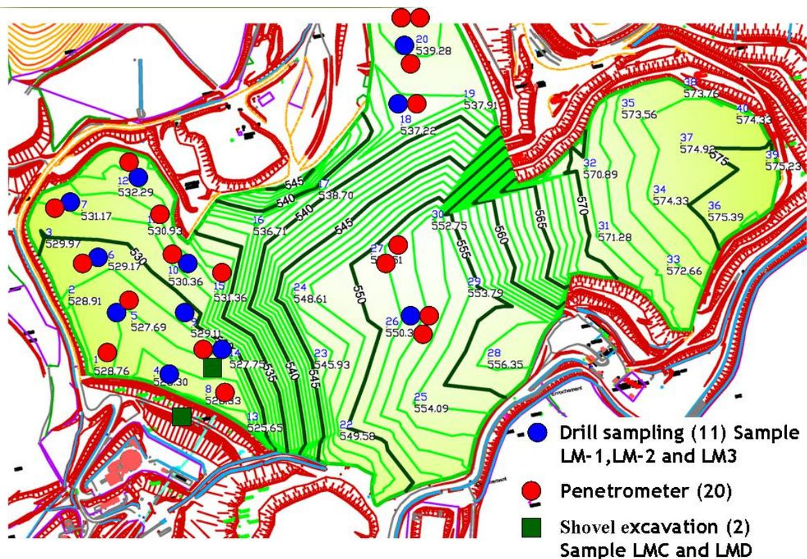
Figure VI- 30: Landfill site ‘LM’ with sample retrieval details.
