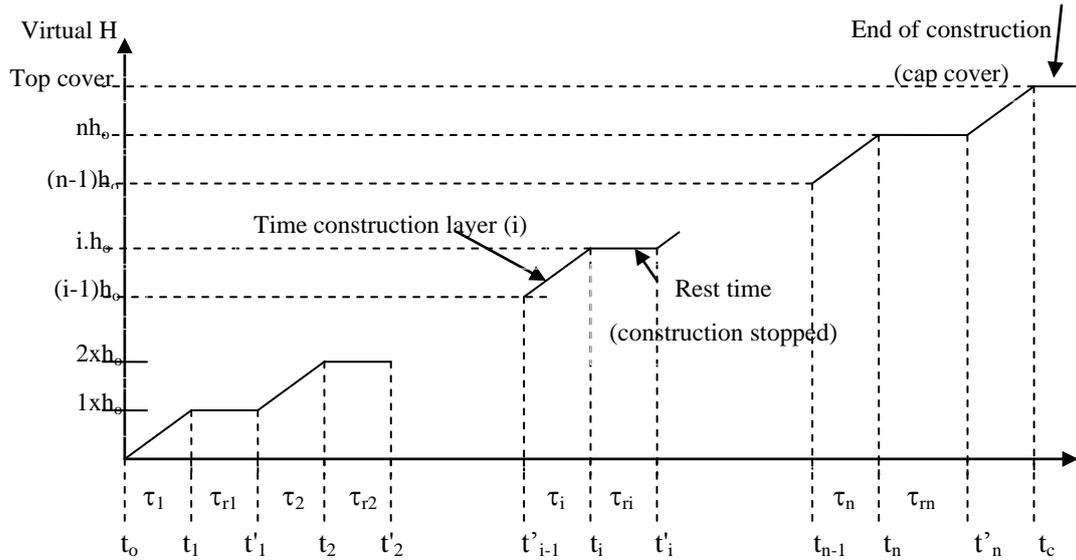
**Figure V- 28: Sequence of construction of the overall landfill.**
