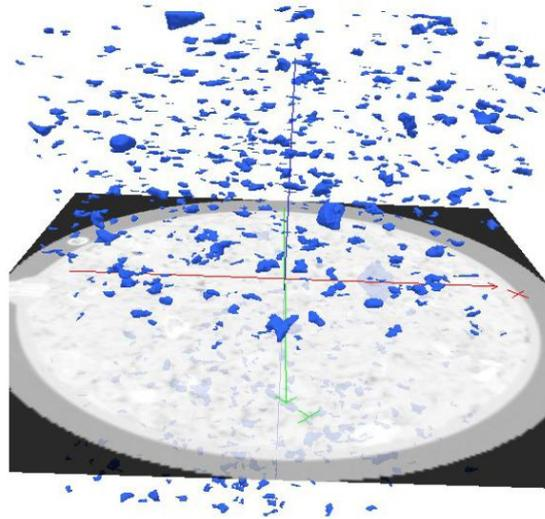
**Figure II- 11: 3D image of reactor 2 after degradation showing only objects with CT number less than -500, corresponding to gas-filled voids. The uniform grey area represents the plane of the centre of the midpoint piezometer port to provide absolute location (Watson et al., 2007).**
