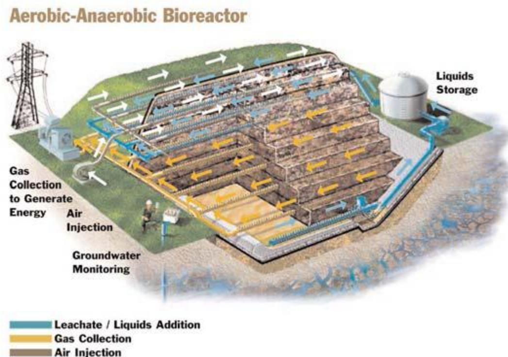
Figure I-22 : Hybrid bioreactor landfill (Waste Management, 2000).
