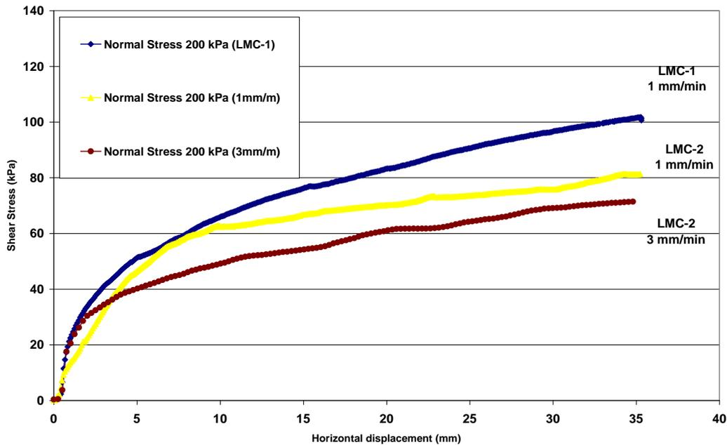
**Graph VI- 9: Comparison of shear behaviour of sample “LMC-2” (shredded saturated and over consolidated at 200 kPa) sheared at 1mm/min and the sample sheared at 3mm/min with the sample LMC-1 which was normally consolidated.**
