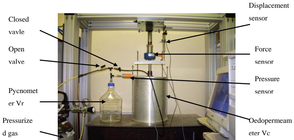
2<sup>nd</sup> Stage: Measurement of relative equilibrium pressure  $p_2$  with connecting valve at open position
