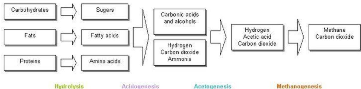
**Figure I-4 : Chemical processes occurring during the four stages of decomposition (Marshal, 2007).**
