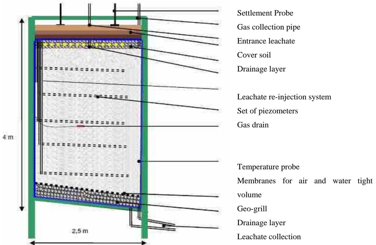
**Figure III- 6: Schematic diagram of the test cell with different systems of devices in place (Lornage, 2006).**
