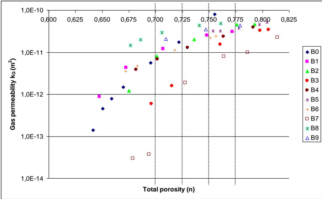
**Graph IV- 2: Change in gas permeability as a function of total porosity of the sample during the compression-gas permeability tests Waste 'B'.**
