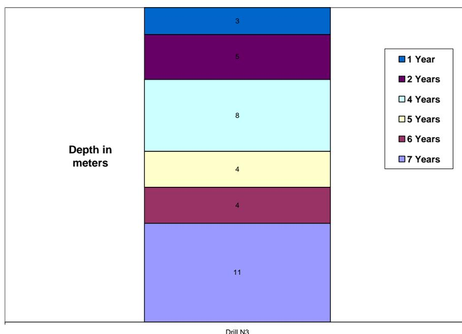
**Figure VI- 45: Age of waste as a function of depth for drilled samples N3.**
