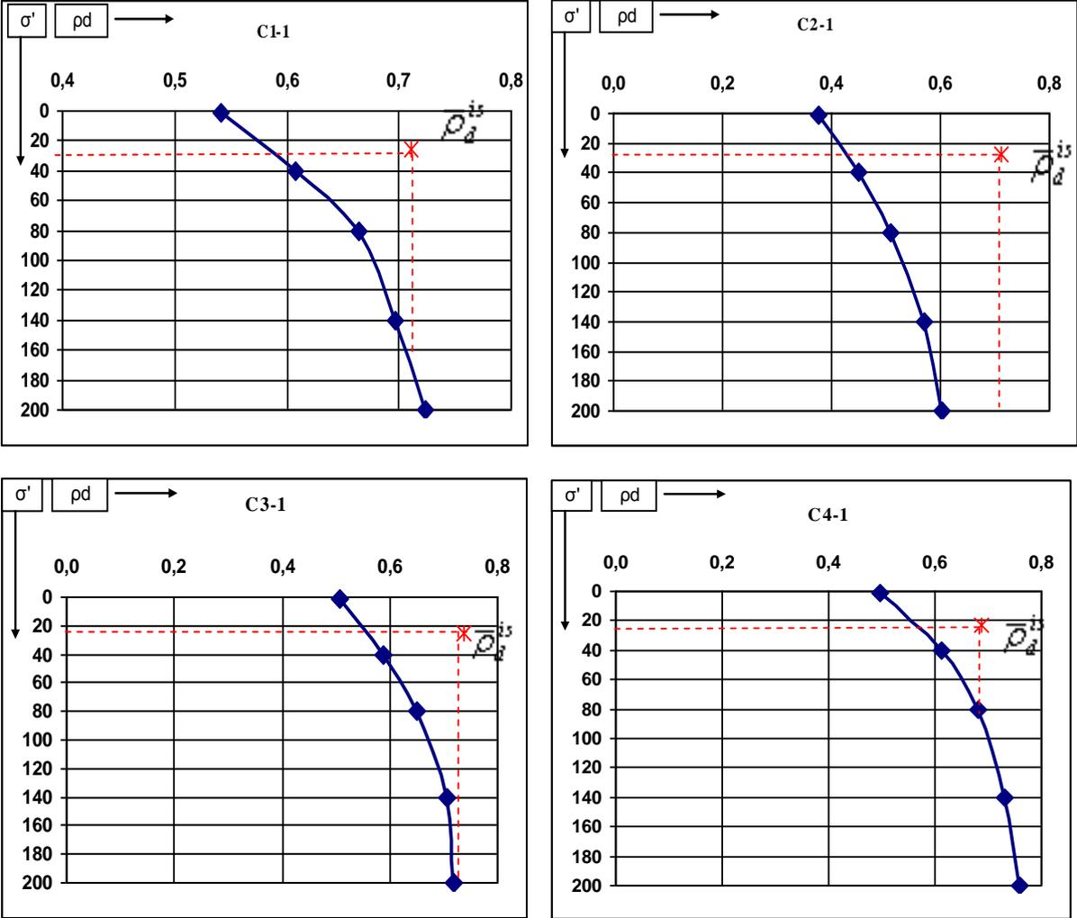
**Graph III- 20: Evolution in dry density ( $\rho_d$ ) of samples (C1-C4) at natural moisture content ( $w_0$ ) as a function of compression stress ( $\sigma$ ) during the compression-permeability test in comparison with the in-situ density ( $\bar{\rho}_d^{is}$ ).**
