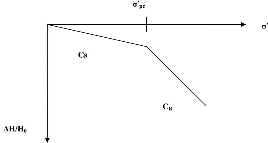
**Figure V- 17: Illustration of the primary consolidation according to the Terzaghi theory (1943).**
