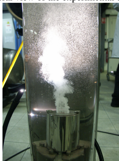
Fig. 3b. Detailed view of gas diffuser
