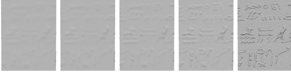
Figure 3.10: Back-projecting the mesh of a single scan of a fine-scale object (engravings are around 0.1mm deep). From left to right: mesh built after 4 scale space iterations; back-projection of the mesh to levels 3, 2, 1; back-projected mesh (final mesh)
