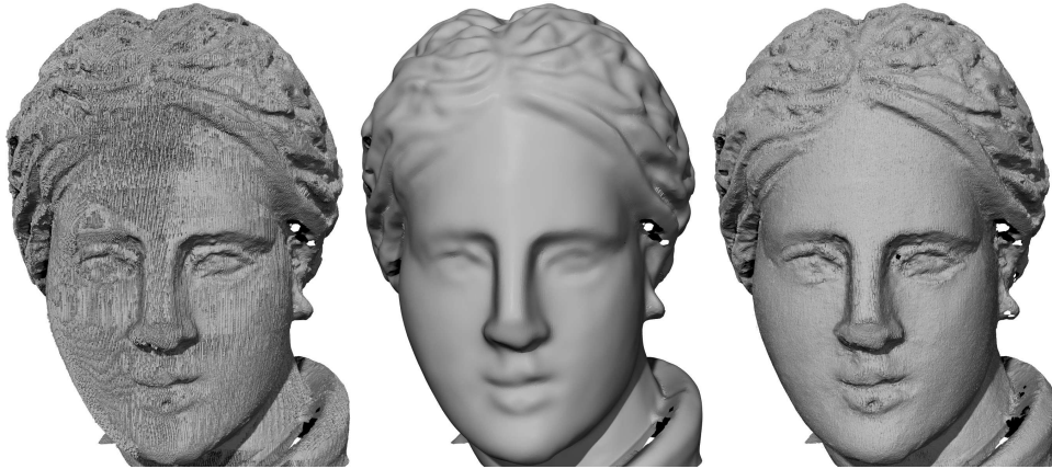
Figure 4.3: The unmerged head with aliasing artifacts (left), its smooth base (middle) and the merged result (right)
