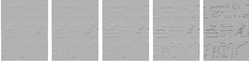
Figure 3.10: Back-projecting the mesh of a single scan of a fine-scale object (engravings are around 0.1mm deep). From left to right: mesh built after 4 scale space iterations; back-projection of the mesh to levels 3, 2, 1; back-projected mesh (final mesh)
