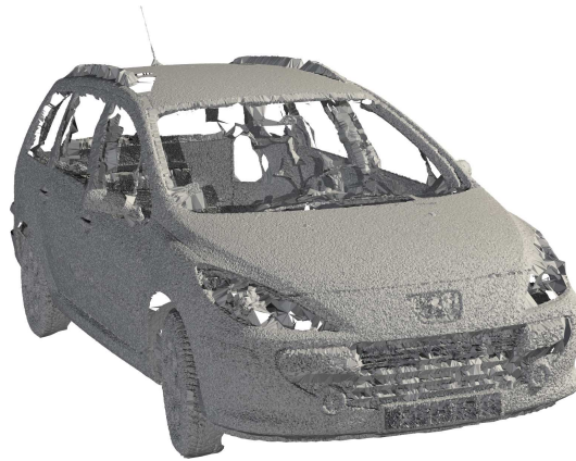
Figure 2.1: A Peugeot car acquired by a range laser scanner (acquisition made by Délégation Générale de l'Armement).
