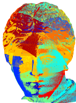
Figure 4.2: Example of overlapping scans. This head is such a complex structure that not less than 35 scans were acquired to fill in most holes.
