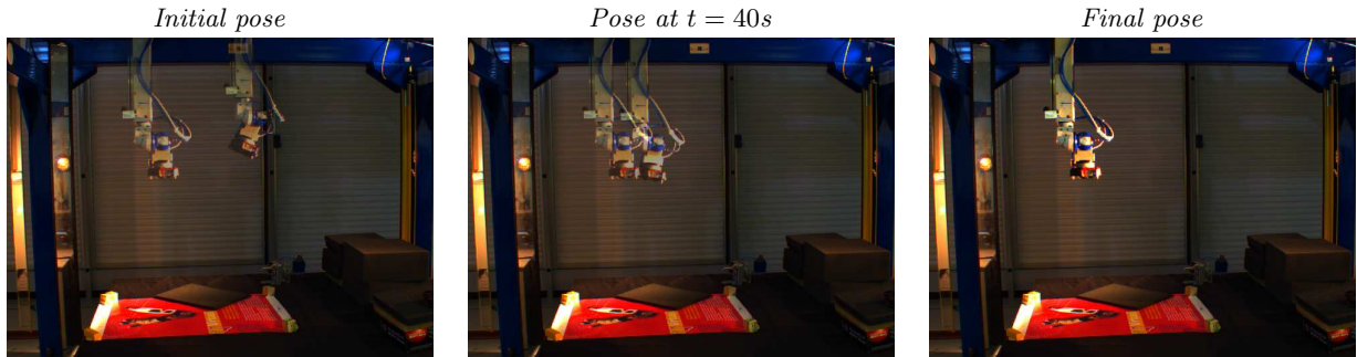
Figure 7.1: External view of one MI-based visual servoing task. The current and desired poses of the robot are overlaid. On the final pose, there is no difference between the two poses.
