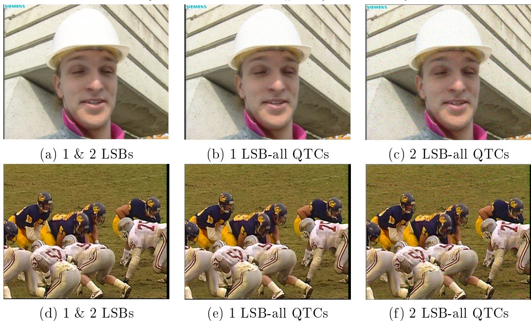
Figure 6.8: Visual comparison of 1 & 2 LSBs mode with naive 1 LSB and 2 LSBs mode (embedding in all QTCs) for intra frame #0 for QP value 18.
