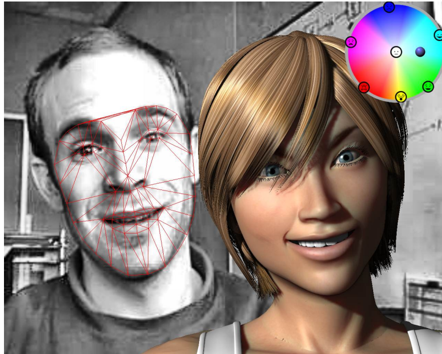
Figure 6.4: The Mimic Game: real-time imitation of emotional facial expressions. The application captures head movements and facial deformations on a human face, interprets these movements as an emotional expression and animates the face of a virtual character to imitate this expression. See the accompanying video for a better demonstration.
