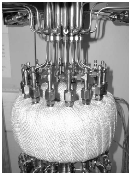
Figure III.9: Catalytic reactor (Spider Reactor) for high throughput testing [8]
