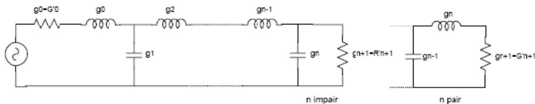
**Fig E. 2. Prototype passe-bas**
