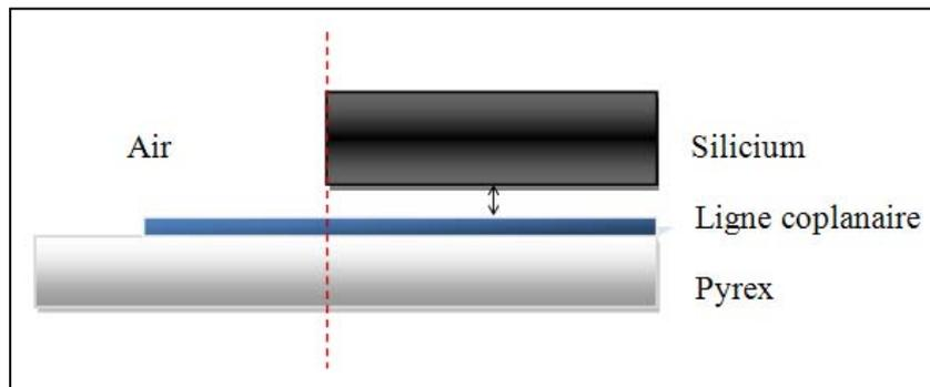
Fig III. 32. Transition air/silicium
