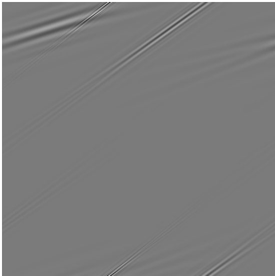
FIG. 4.4: a) Image reconstruction of three curvelet coefficients. b) The discrete FFT of the image a).
